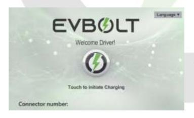
Simply plug in the charger to the vehicle and tap the screen to proceed.
