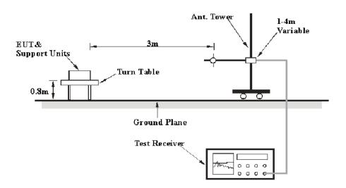
The radiated emission tests were performed in the 3-meter chamber a test site, using the setup accordance with the ANSI C63.10-2013.
