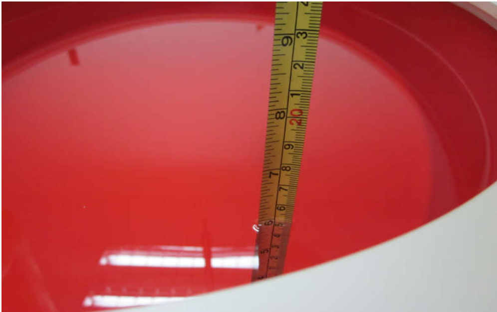
Figure 4.4: Liquid depth in the Flat Phantom
