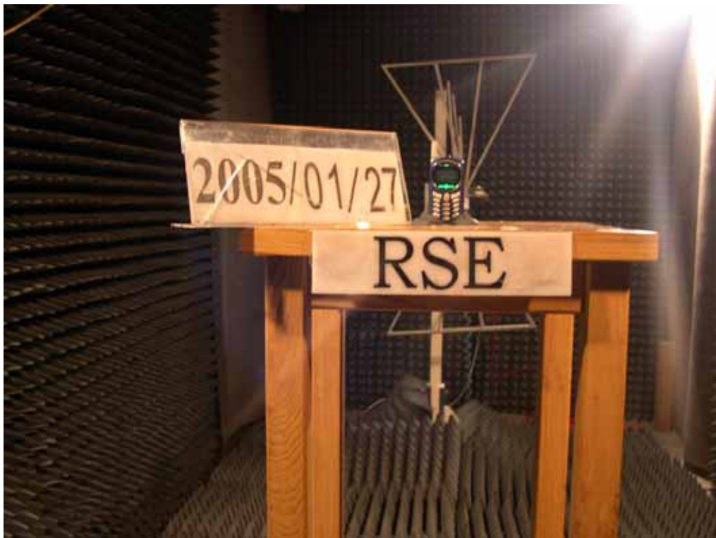
TCL558 Radiated Spurious Emission Test Setup
