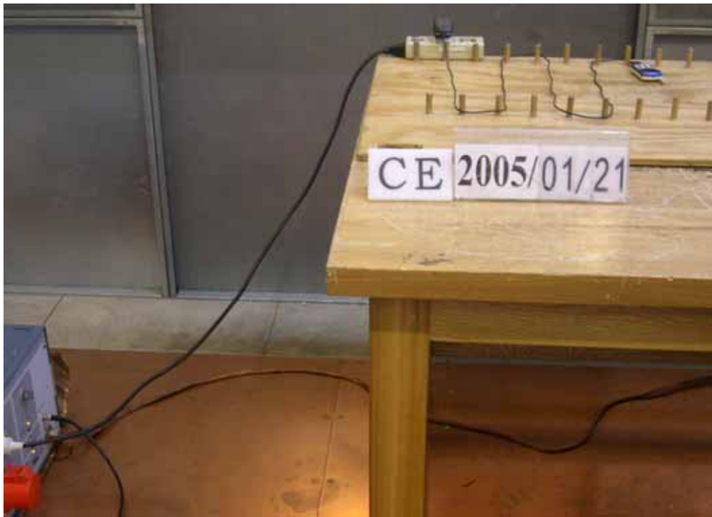
TCL558 Conducted Emission Test Setup
