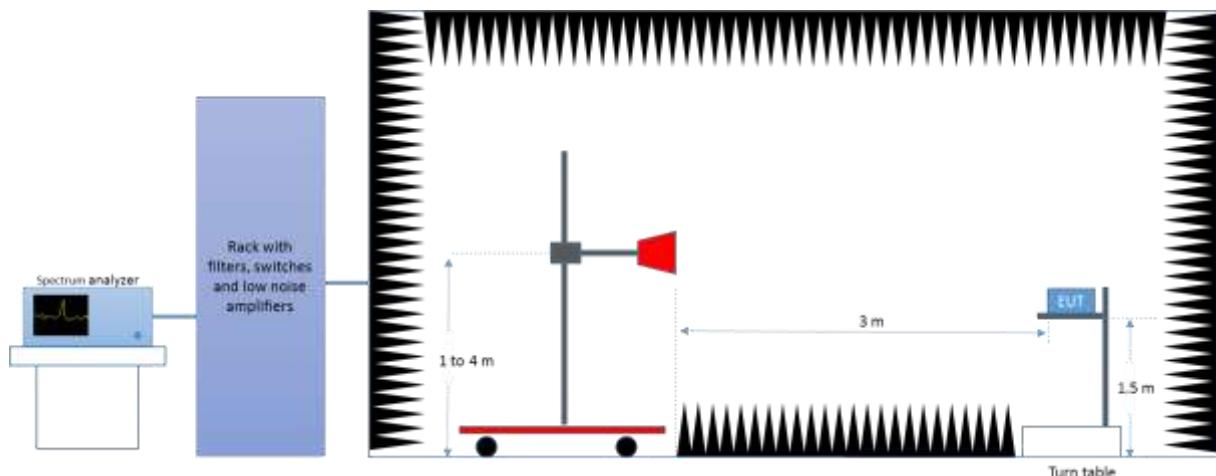
*Radiated Setup 6.4 GHz – 18 GHz*
