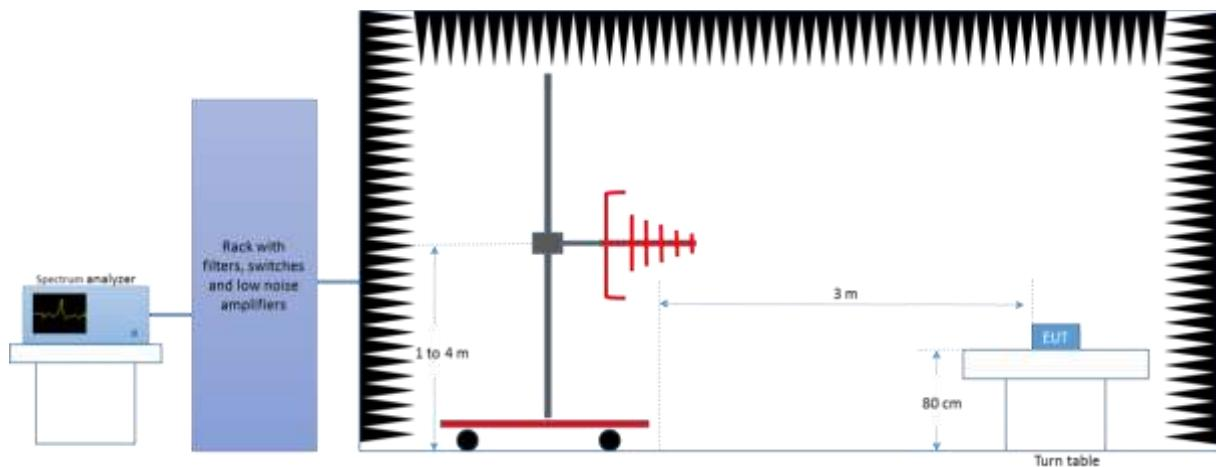
*Radiated Setup 1 GHz – 6.4 GHz*
