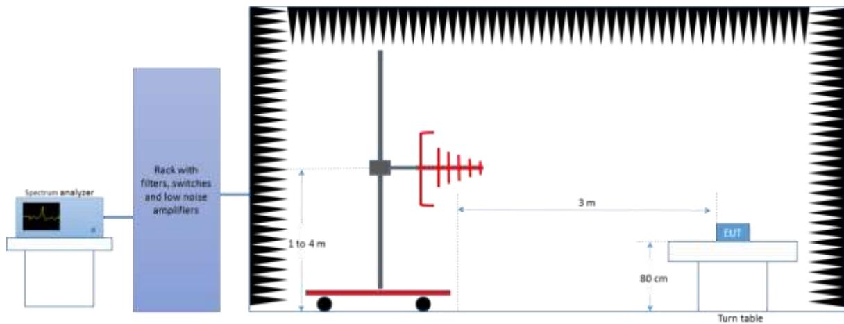
*Radiated Setup 1 GHz – 6.4 GHz*
