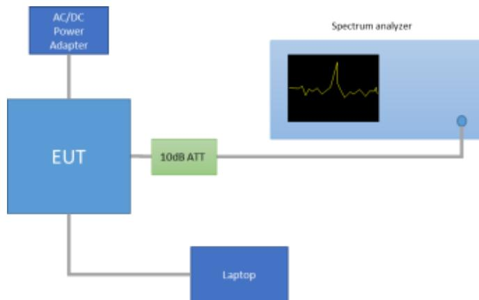
For Band Edge measurements in average mode on the low frequency section, one of the two methods is used according to section G) 6) (KDB 789033 D02):
