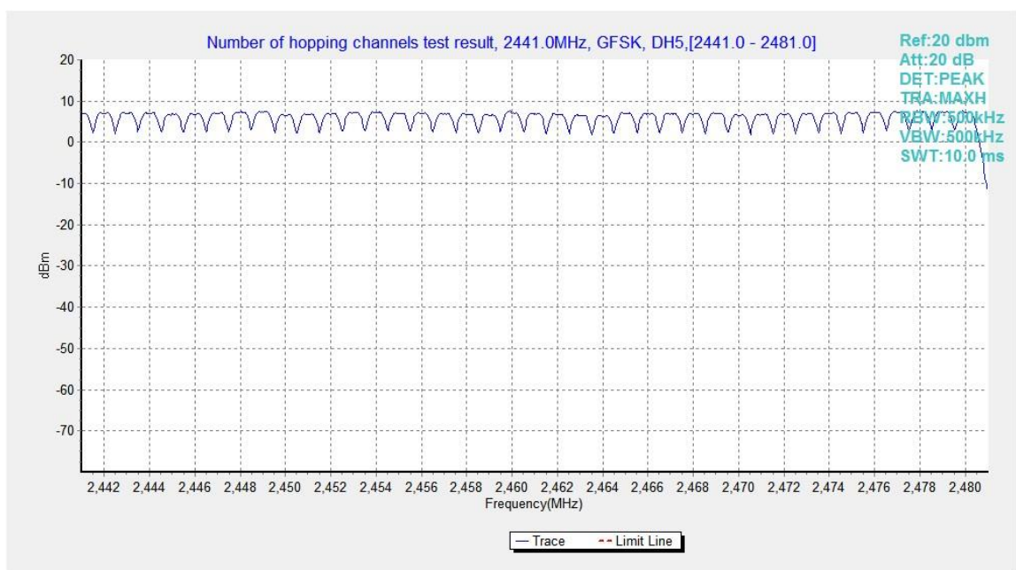
Fig.95. Number of hopping frequencies: GFSK, Channel 40 - 78
