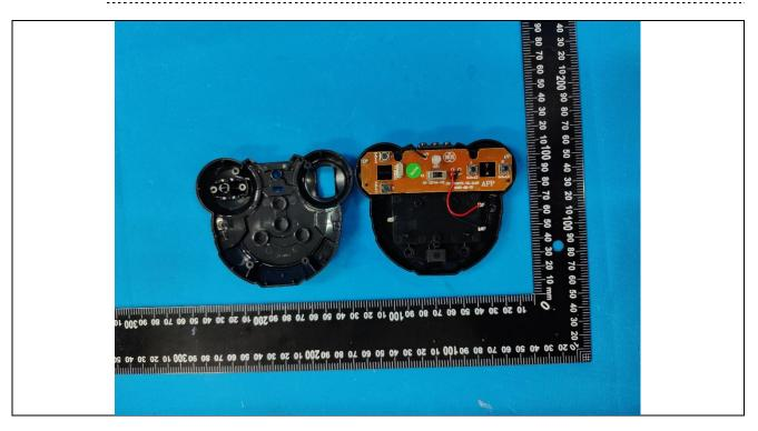
Details of: PCB view for Remote controller
