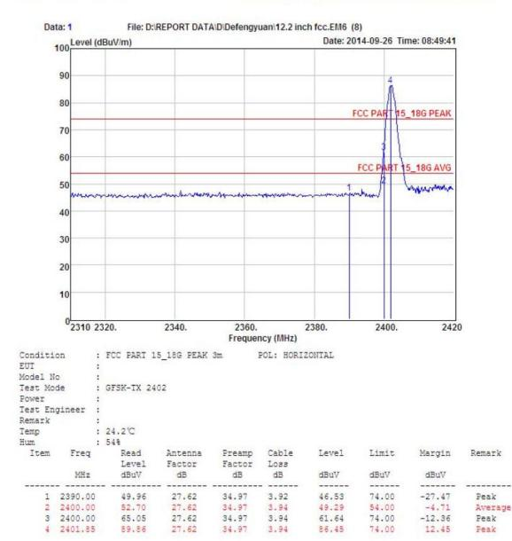
Remark: Level = Read Level + Antenna Factor - Preamp Factor + Cable Loss
