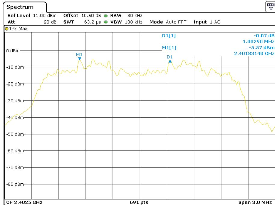
**EDR (8DPSK): Middle Channel**
