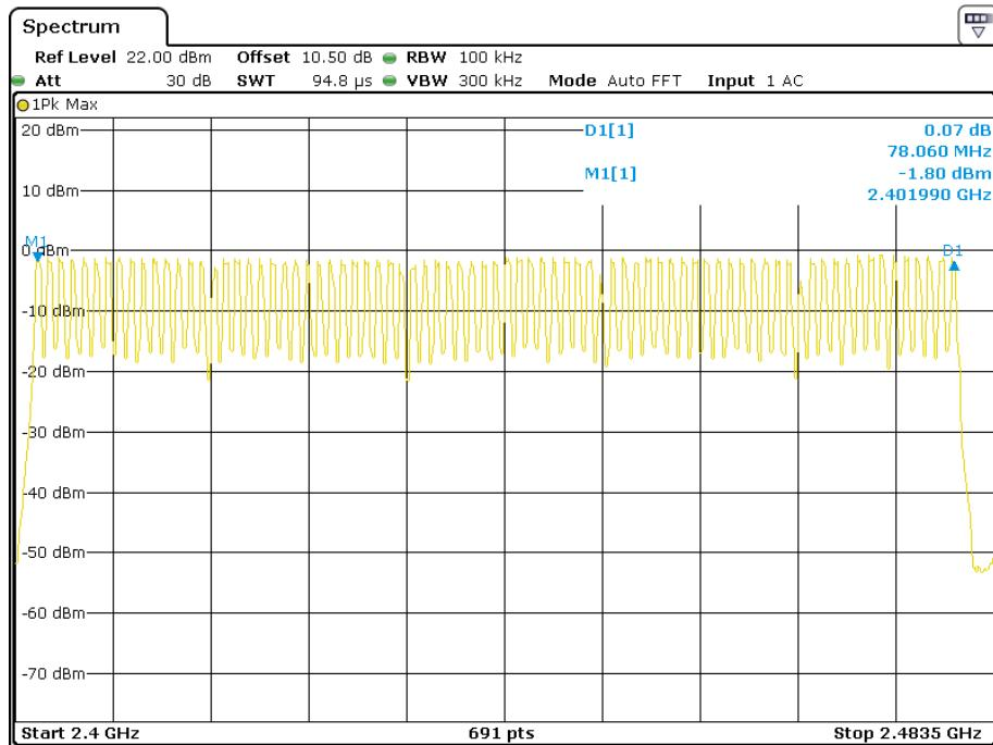
**EDR ( $\pi/4$ -DQPSK): Number of Hopping Channels**
