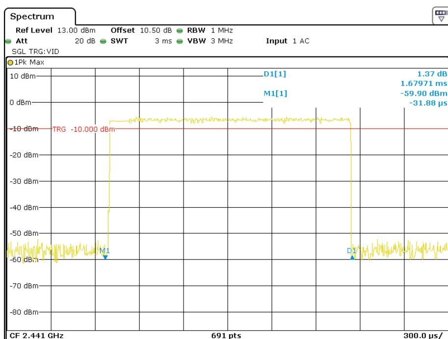
**Pulse time, High Channel, 2DH3**
