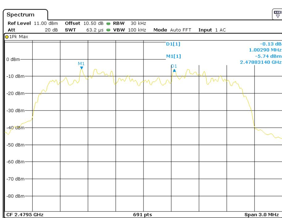
**EDR (8DPSK): Low Channel**
