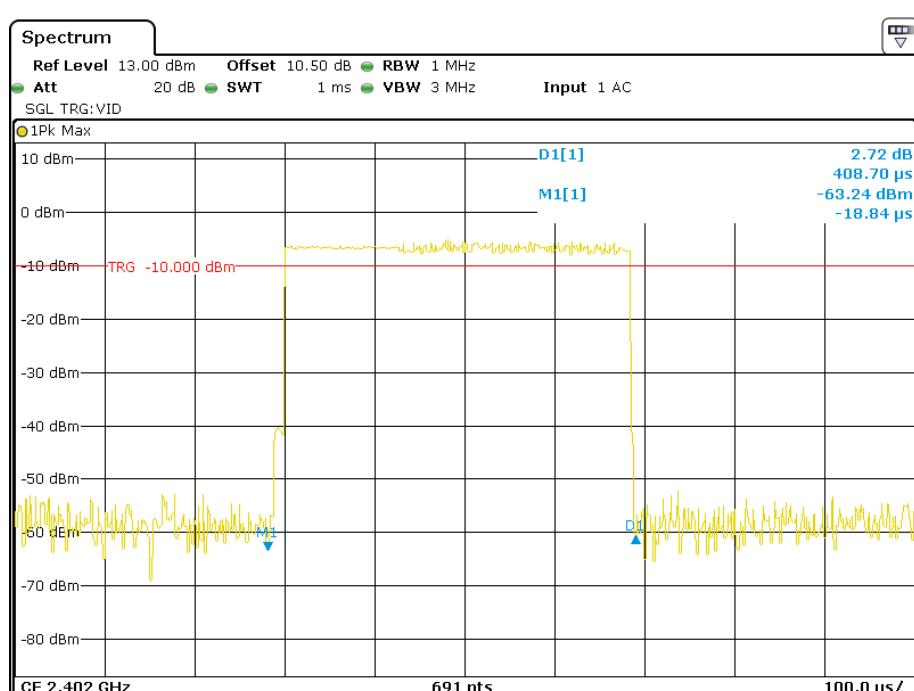
**Pulse time, Middle Channel, 2DH1**
