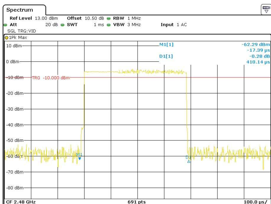
**Pulse time, Low Channel, 2DH3**
