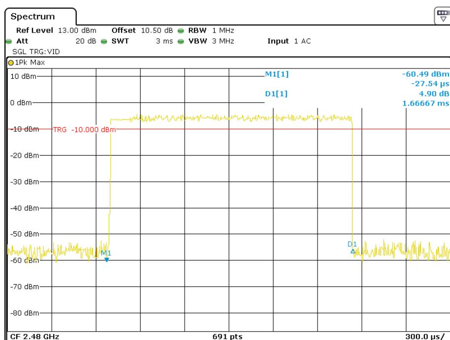
**Pulse time, Low Channel, 3DH5**
