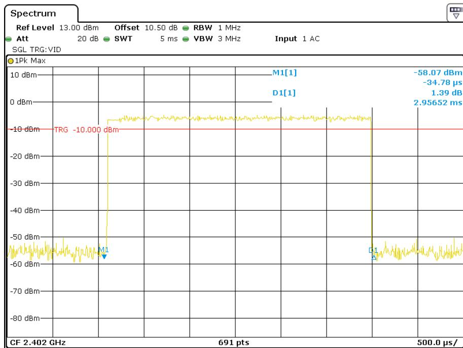
**Pulse time, Middle Channel, 3DH5**
