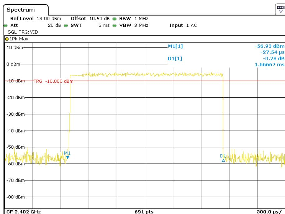
**Pulse time, Middle Channel, 3DH3**
