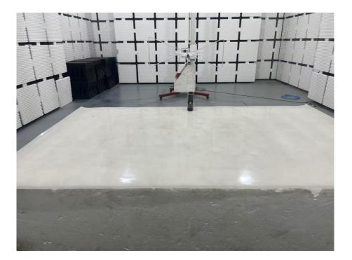
Set-up for Radiated Spurious Emission, Below 1GHz
