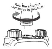
Caution: Do not hold the radio by its antenna, otherwise the performance and lifespan of the antenna will be reduced.
