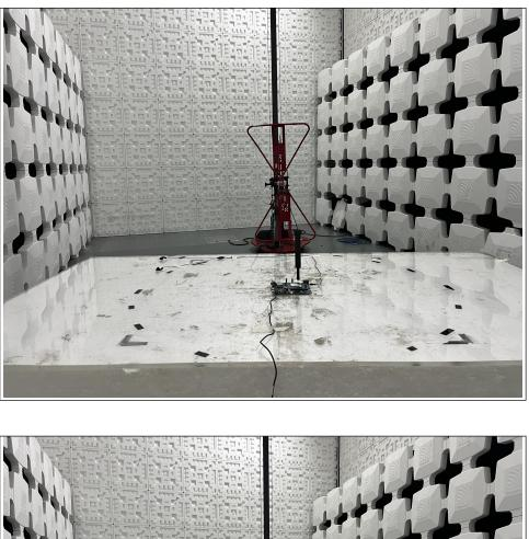
Radiated emission test: Frequency Range< 30MHz ~1GHz >
