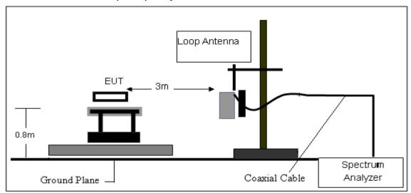
2. Radiated Emission Test-Up Frequency 30MHz~1GHz
