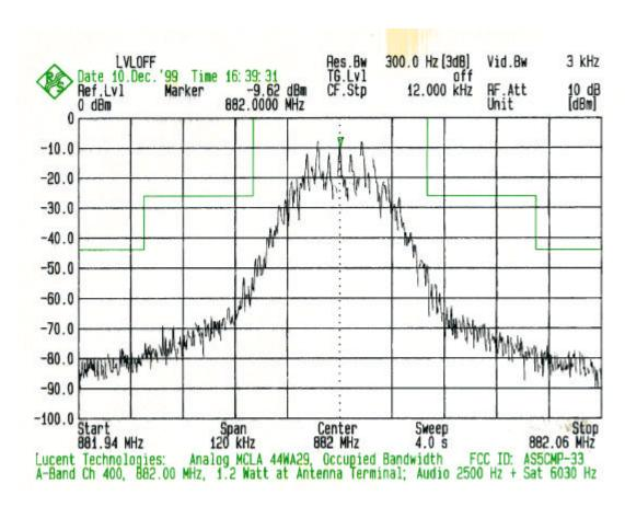
PLOT # 13 Output: Ch 400 + Audio at 2500 Hz + SAT at 6030 Hz
