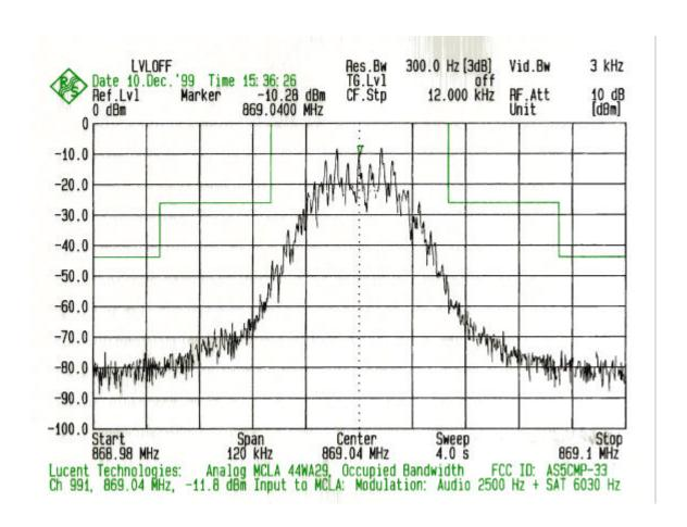
PLOT # 6 Input: Ch 991 + Audio at 2500 Hz + SAT at 6030 Hz
