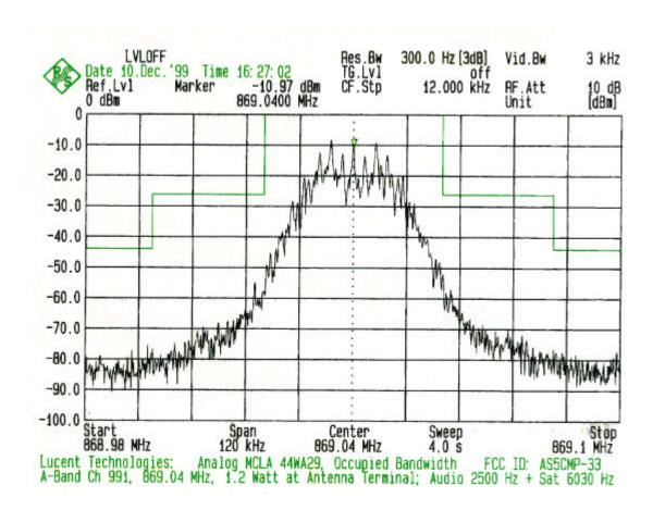
PLOT # 5 Output: Ch 991 + Audio at 2500 Hz + SAT at 6030 Hz
