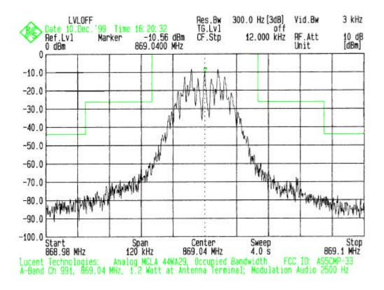
PLOT #1 Output: Ch 991 + Audio at 2500 Hz
