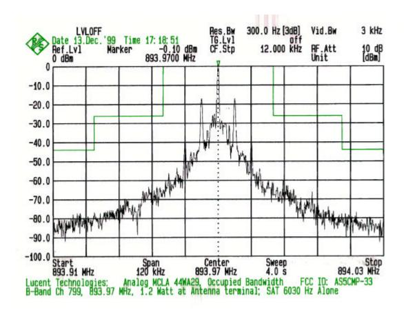
PLOT # 19 Output: Ch 799 + SAT at 6030 Hz
