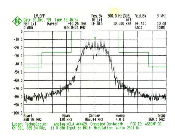
PLOT # 2 Input: Ch 991 + Audio at 2500 Hz
