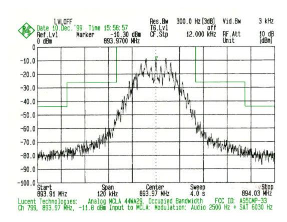
PLOT # 22 Input: Ch 799 + Audio at 2500 Hz + SAT at 6030 Hz
