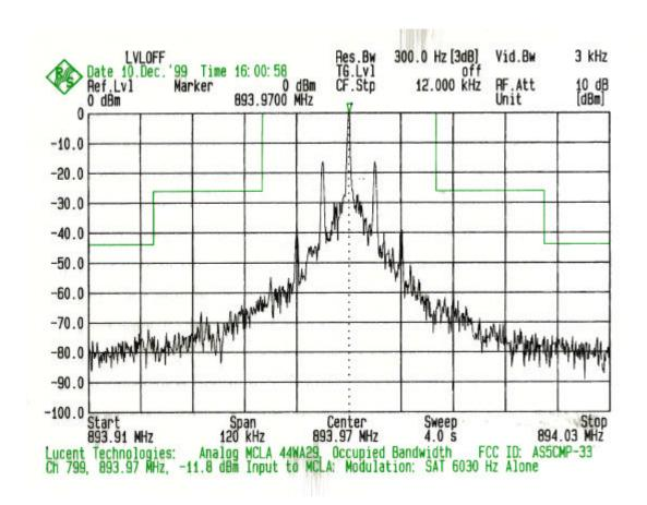
PLOT # 20 Input: Ch 799 + SAT at 6030 Hz
