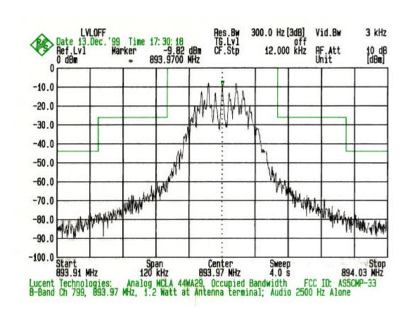
PLOT # 17 Output: Ch 799 + Audio at 2500 Hz
