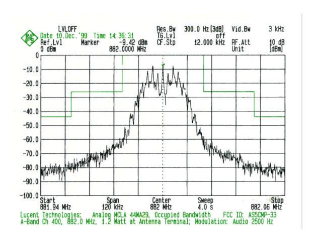
PLOT # 9 Output: Ch 400 + Audio at 2500 Hz
