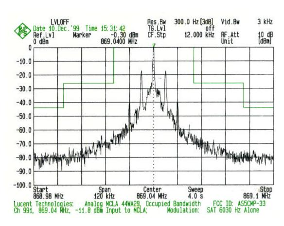
PLOT # 4 Input: Ch 991 + SAT at 6030 Hz
