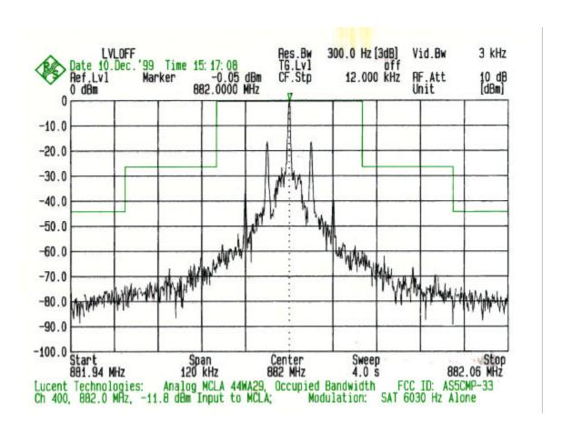
PLOT # 12 Input: Ch 400 + SAT at 6030 Hz
