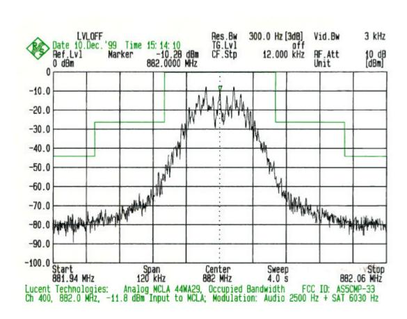
PLOT # 14 Input: Ch 400 + Audio at 2500 Hz + SAT at 6030 Hz
