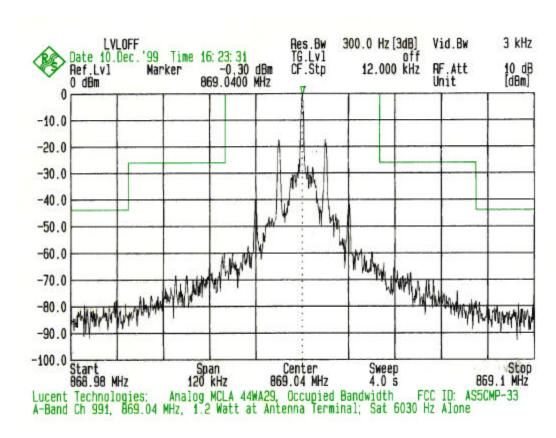
PLOT # 3 Output: Ch 991 + SAT at 6030 Hz APPLICANT: Lucent Technologies FCC ID: AS5CMP-33
