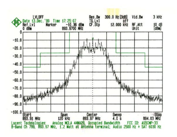
PLOT # 21 Output: Ch 799 + Audio at 2500 Hz + SAT at 6030 Hz
