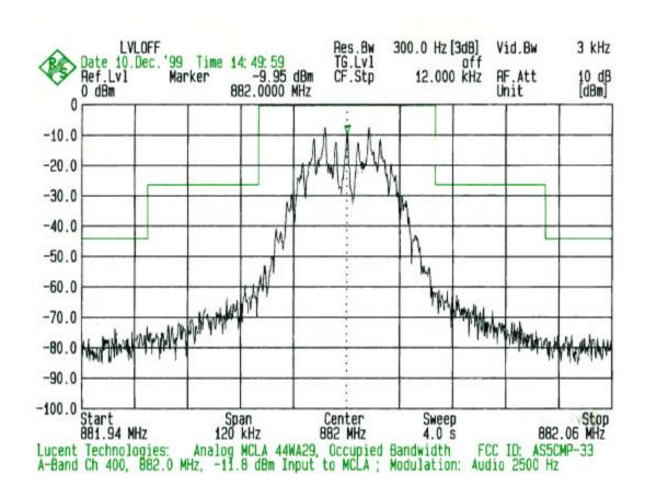
PLOT # 10 Input: Ch 400 + Audio at 2500 Hz
