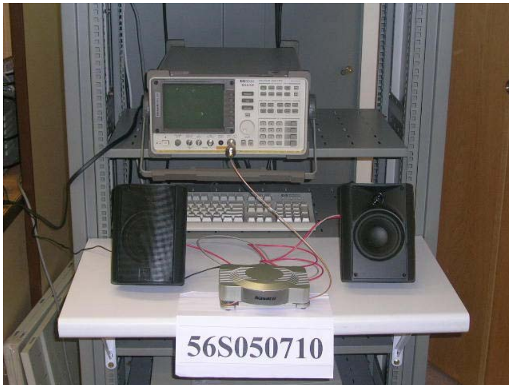
Average Frequency Dwell Time Test Setup
