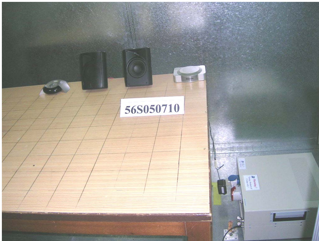
Conducted Emissions Test Setup (Front View)
