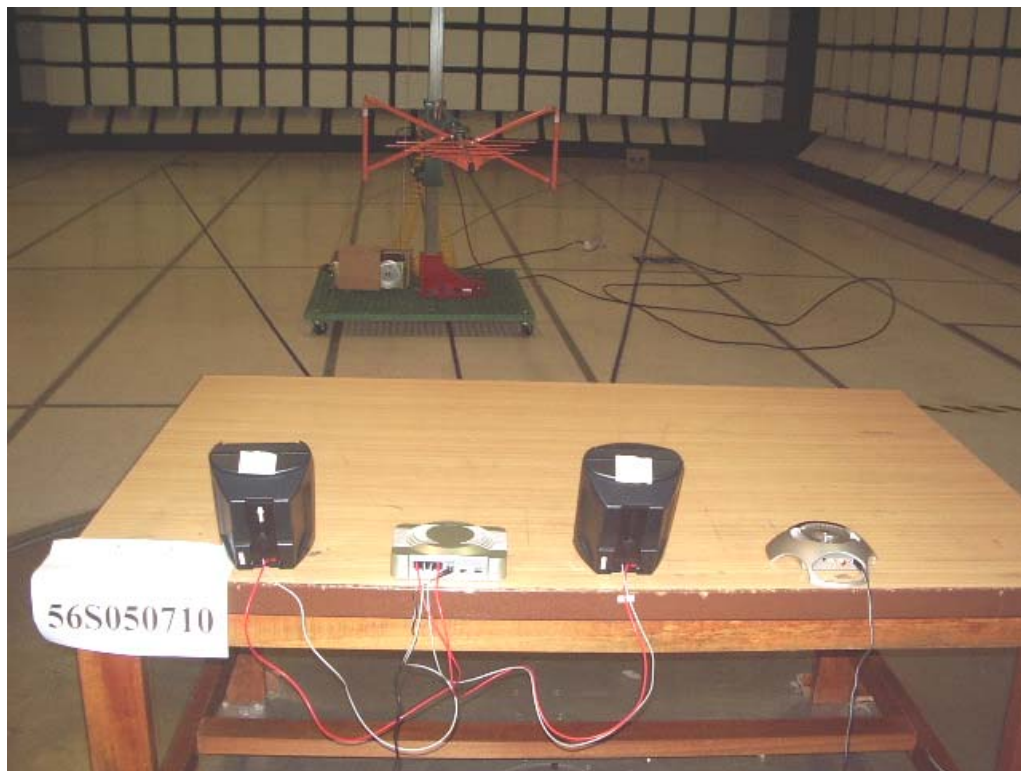
Radiated Emissions Test Setup (Rear View)
