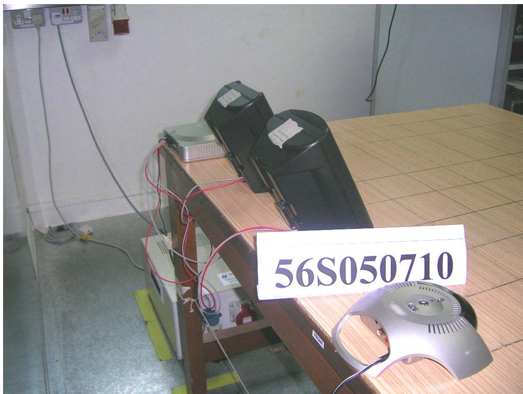
Conducted Emissions Test Setup (Rear View)
