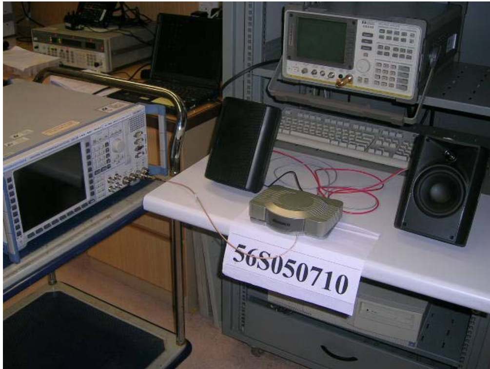
Maximum Peak Power Test Setup
