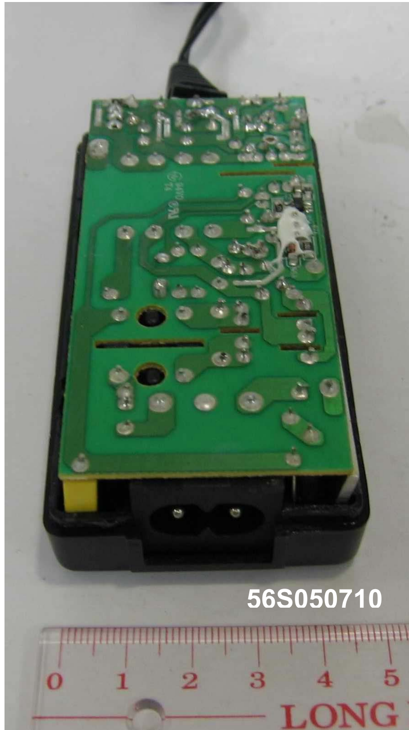
EUT PCB Trace Side
