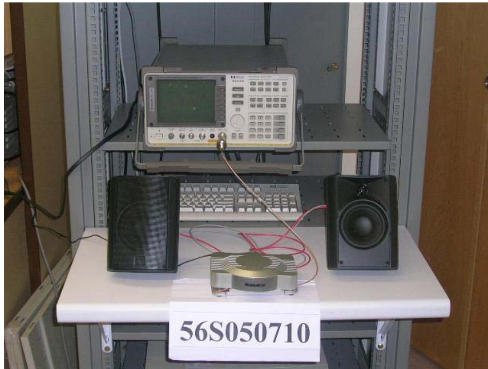
Spectrum Bandwidth (20dB Bandwidth Measurement) Test Setup
