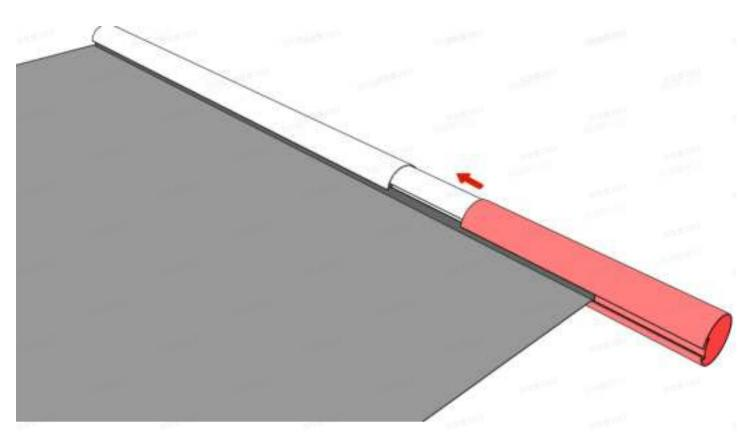
Loosen the screws on the Shade Tube and adjust the size to fit the fabric. (Make sure the fabric on both sides is aligned.)
