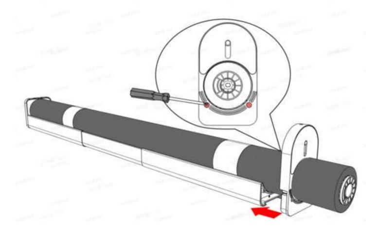
2. Place the Headrail as shown. Tap Start via our app to start the Cutter. Then insert a screwdriver in the top port and rotate counterclockwise.
