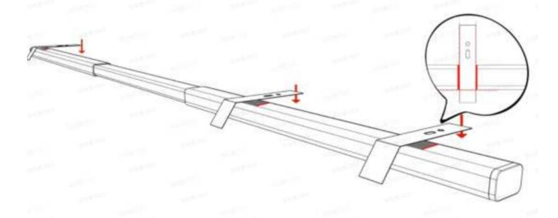
Stick the level to the middle position of the adjusted Bottom Bar, ensuring that the edge of the level is flush with the Bottom Bard edge.
