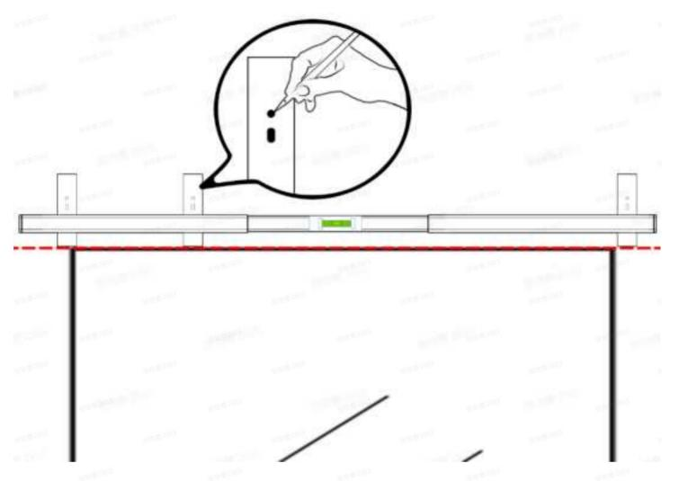
4. Use a handheld electric drill with a drill bit diameter of 5.6-6.0 mm to drill along the marked hole positions, and install expansion anchors.
