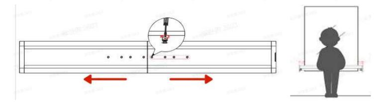
2. Take out the Bottom Bar and adjust it to the same length as the Headrail.
