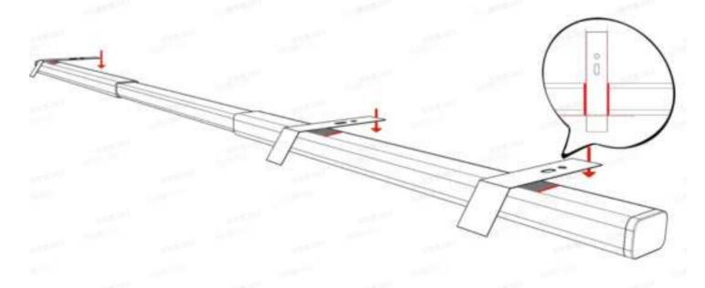
The top part of the positioning card should not protrude beyond the outer edge of the window.
