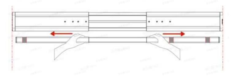
3. Tear off the tape liner on the positioning cards and attach them to the Bottom Bar as shown.
