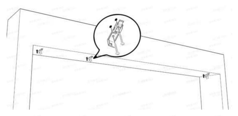
6. Install the adjusted Headrail onto the brackets, check if the brackets are properly positioned, and then remove the Headrail.
