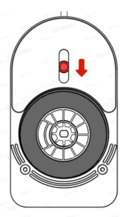
If the fabric is stuck and the cutting is not finished, rotate the screwdriver clockwise for 1 to 2 circles and start the Cutter via our app to try again.
