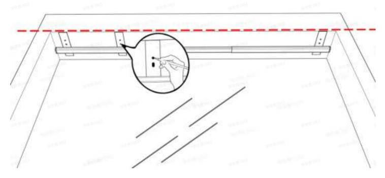
4. Use a handheld electric drill with a drill bit diameter of 5.6-6.0 mm to drill along the marked hole positions, and install expansion anchors.
