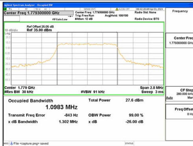
B66 / 1.4MHz / 64QAM/ High CH
