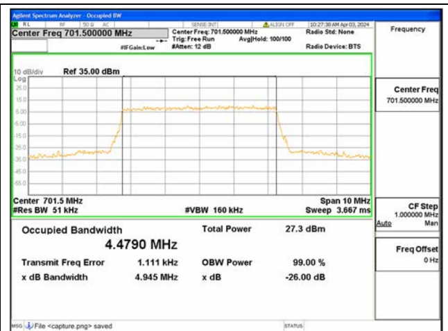
B12 / 5MHz / 16QAM/ Low CH
