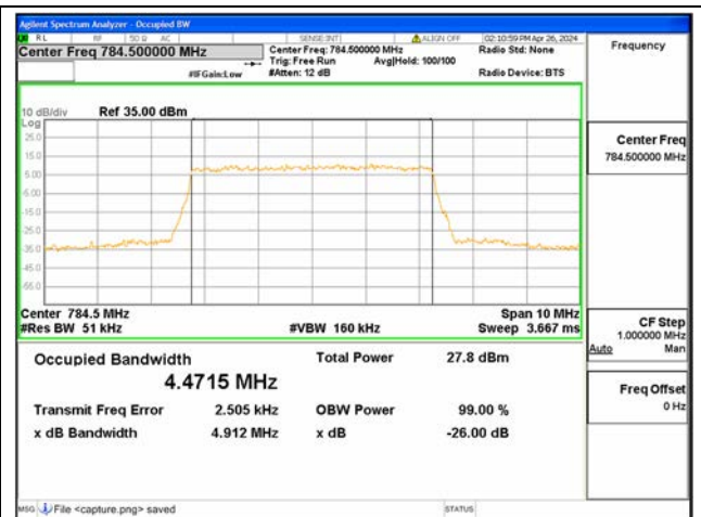
B13 / 5MHz / 16QAM/ High CH
