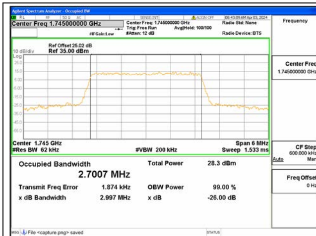
B66 / 3MHz / QPSK/ Mid CH
