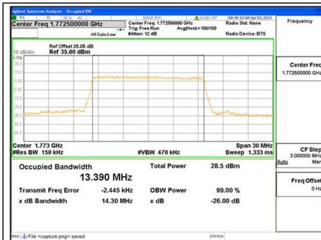
B66 / 15MHz / QPSK/ High CH
