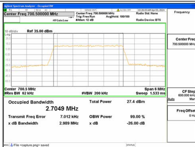
B12 / 3MHz / 16QAM/ Low CH
