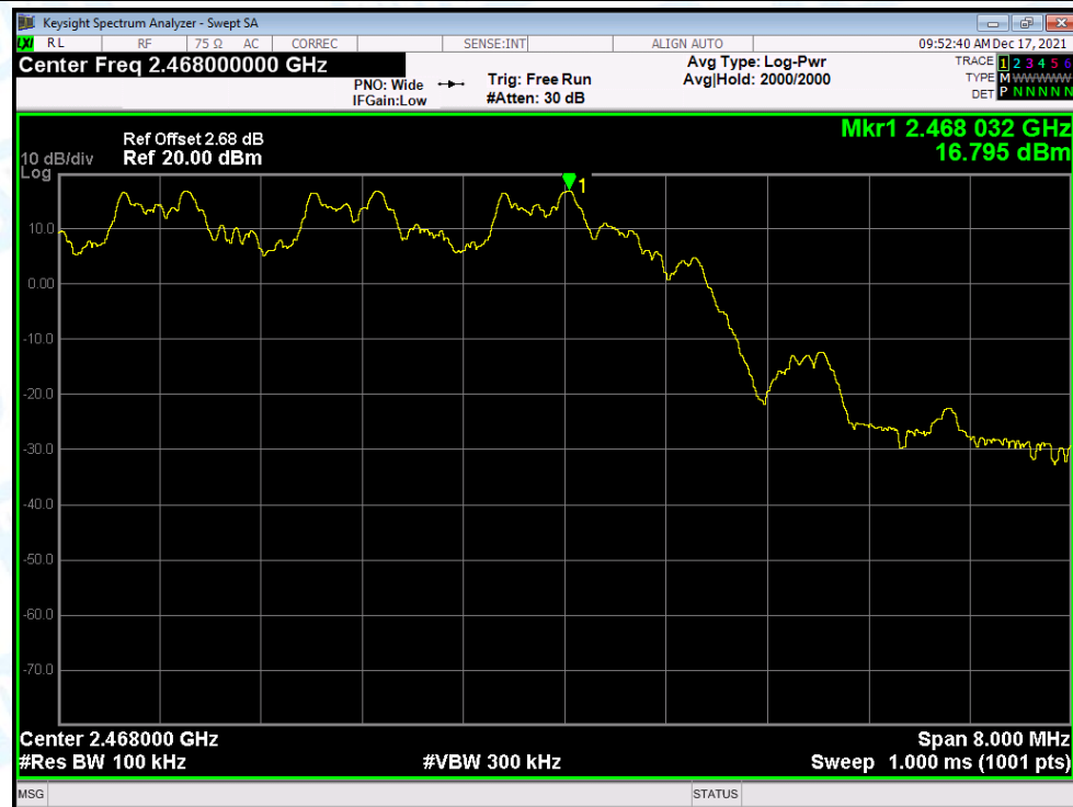
Band Edge(Hopping) NVNT user 2468MHz Ant1 Hopping Emission
