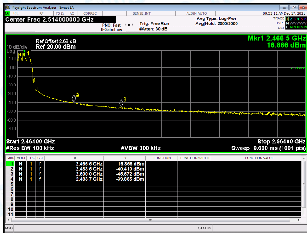
Band Edge(Hopping) NVNT user 2468MHz Ant1 Hopping Emission
