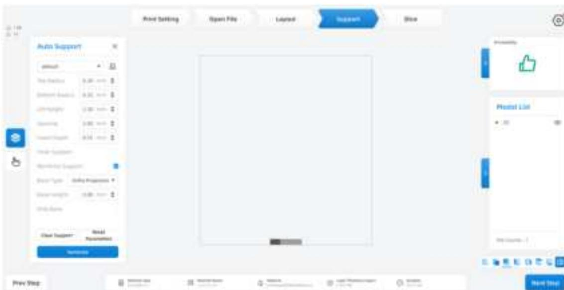
AccuWare supports Auto support and Manual support. User can add support Manually or generate Automatically by the support settings.
