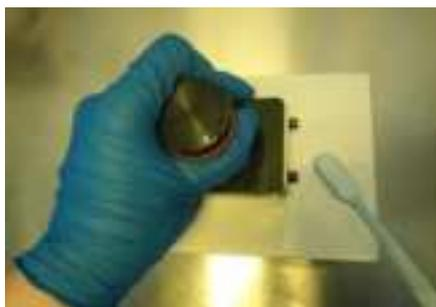
Step 3 Dry the surface of the build platform with a paper towel, and dry in a ventilated place before reuse.
