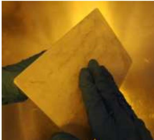
Step 2 Use the soft glue brush with wet alcohol to clean up the residual resin on the surface of the build platform.
