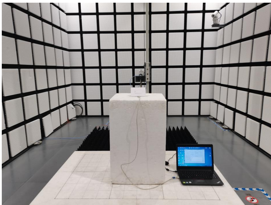
Fig. 3 Radiated emission setup photo(Above 1GHz)
