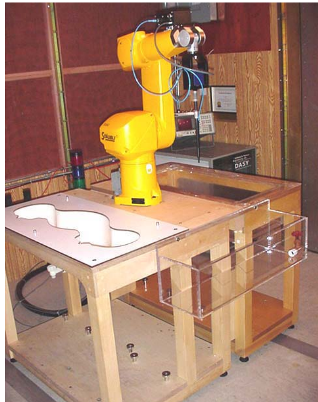
DASY4 SAR Measurement System with Plexiglas planar phantom
