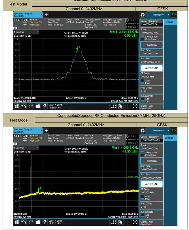
Bluetooth (GFSK, pi/4-DQPSK,8DPSK) mode have been tested, and the worst result(GFSK)was report as below: Maximum Conduceted Level RBW=100kHz
