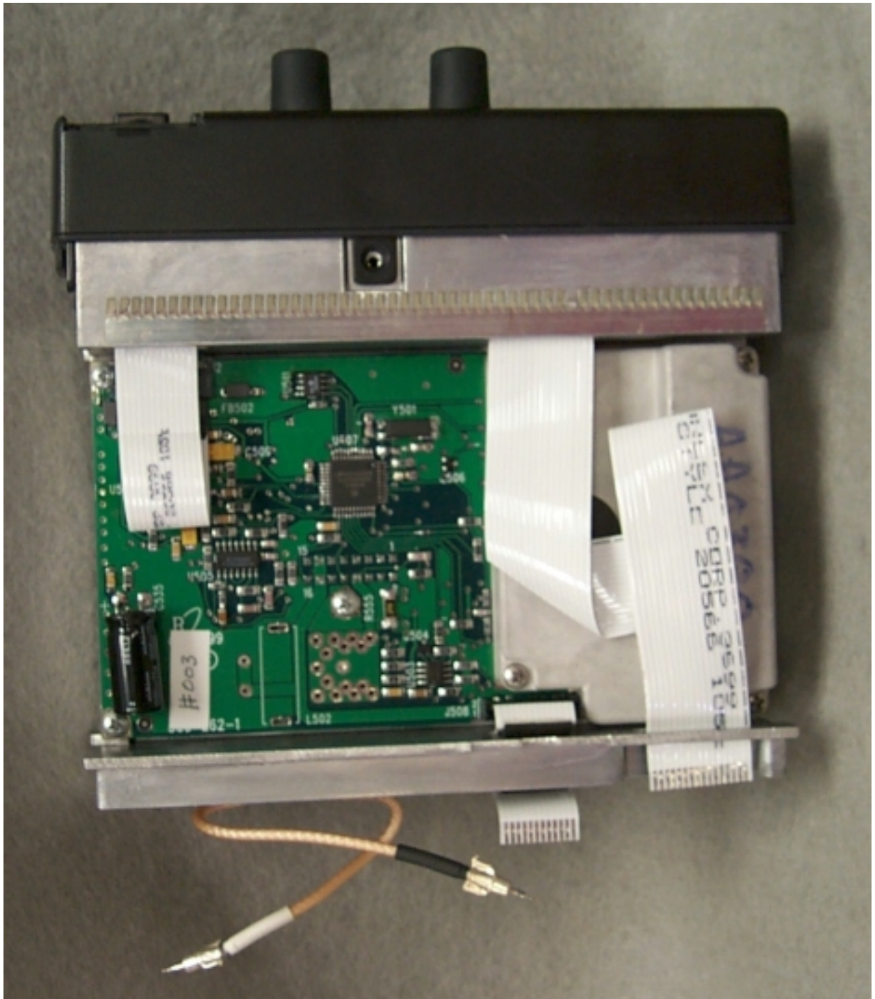
Photo 9. EUT, Bottom View of Main Chassis with Case Removed Showing System Board
