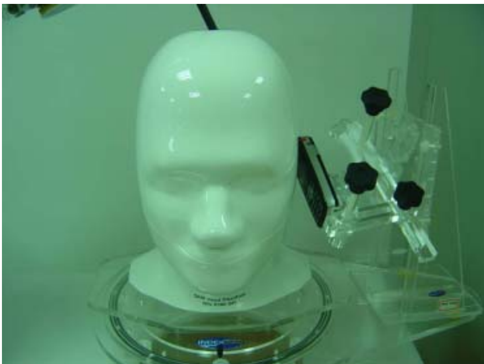
Fig.4 EUT Left Head Tilt15 Position
