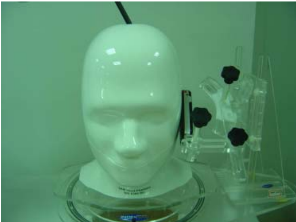
Fig.3 EUT Left Head Touch Cheek Position
