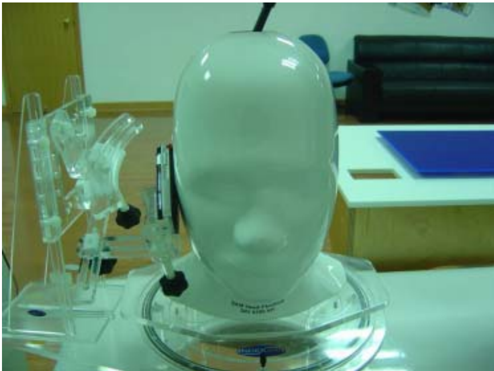
Fig.5 EUT Right Head Touch Cheek Position
