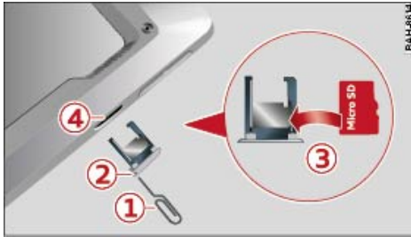
Fig. 28 Rear side of Audi tablet: Changing micro SD card
