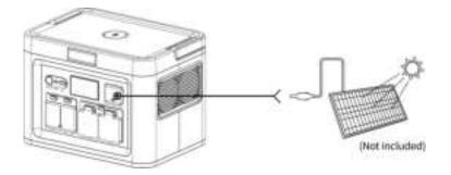
$\triangle$  The total open circuit voltage of solar modules after series-parallel connection should not exceed the specified voltage! please confirm the same voltage specification.
