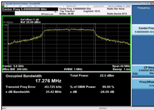
U-NII-2c 99%&26dB Bandwidth-802.11a(20MHz) ,5600MHz,Ant0
