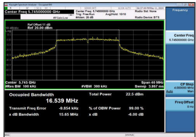
U-NII-3 6dB Bandwidth-802.11a(20MHz) ,5745MHz,Ant0
