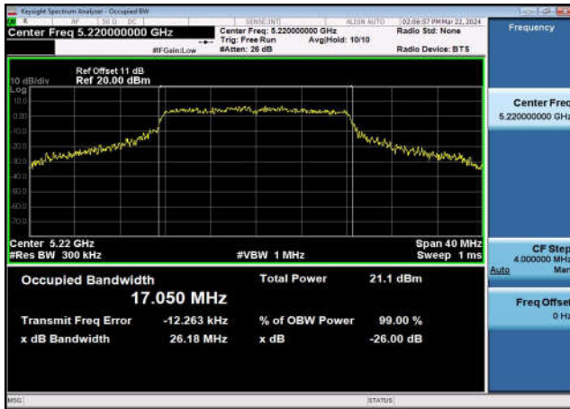
U-NII-2c 99%&26dB Bandwidth-802.11a(20MHz) ,5600MHz,Ant0
