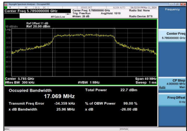
U-NII-3 99%&26dB Bandwidth-802.11a(20MHz) ,5785MHz,Ant0
