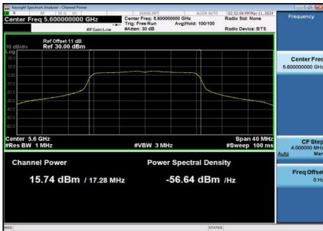
U-NII-2c Output Power-802.11a(20MHz) ,5600MHz,Ant0
