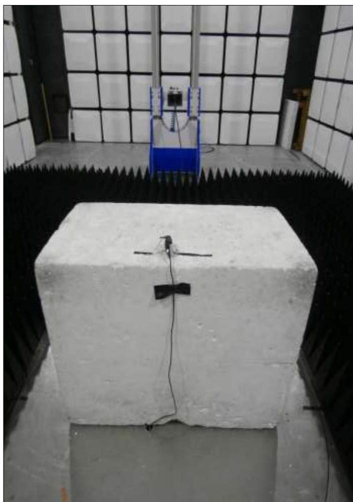
Figure 29 - Test Setup - 1 GHz to 13 GHz - Z Orientation
