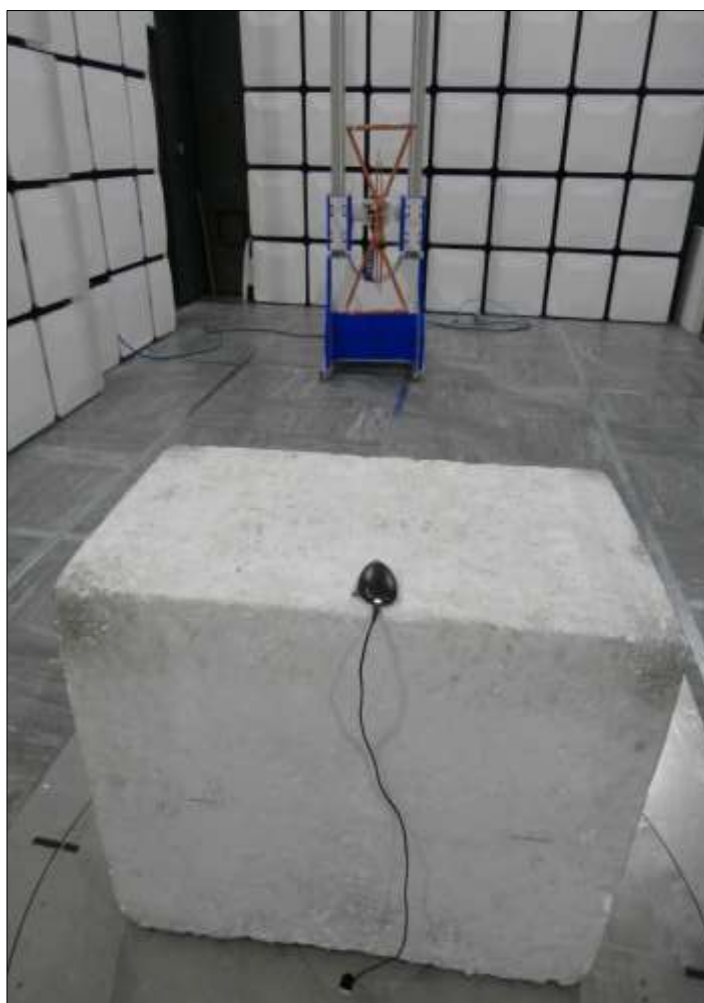
Figure 24 - Test Setup - 30 MHz to 1 GHz - X Orientation
