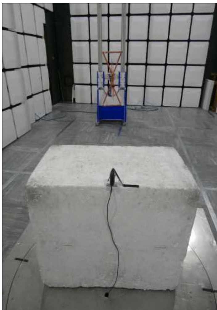
Figure 28 - Test Setup - 1 GHz to 13 GHz - Y Orientation
