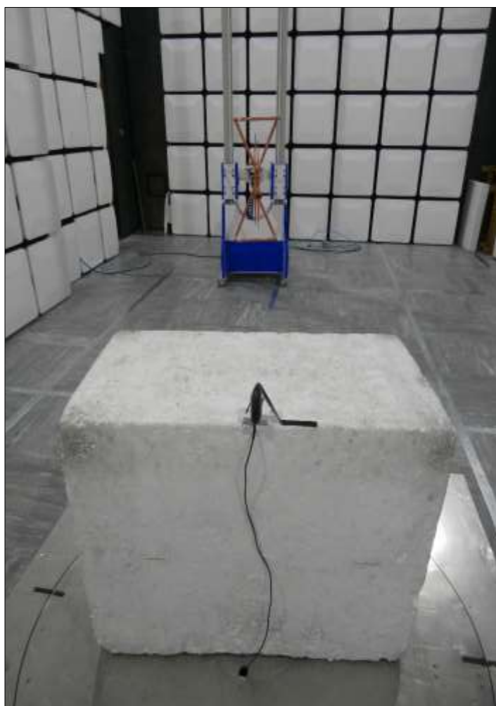
Figure 25 - Test Setup - 30 MHz to 1 GHz - Y Orientation
