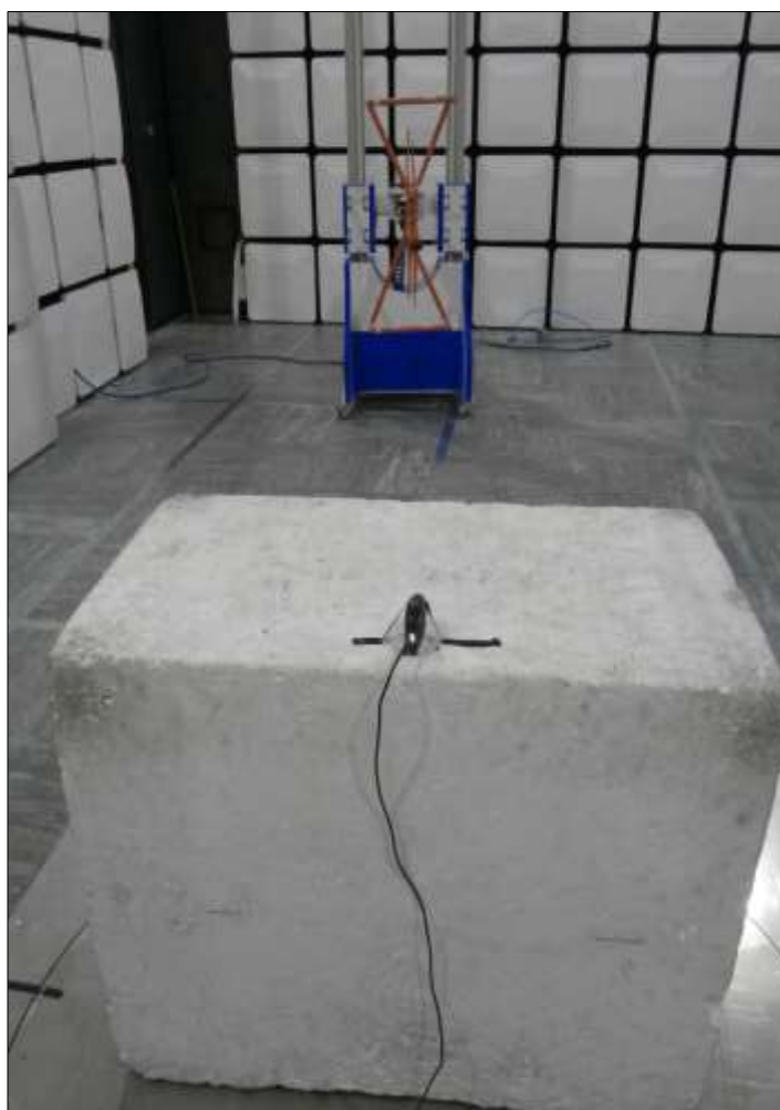
Figure 26 - Test Setup - 30 MHz to 1 GHz - Z Orientation
