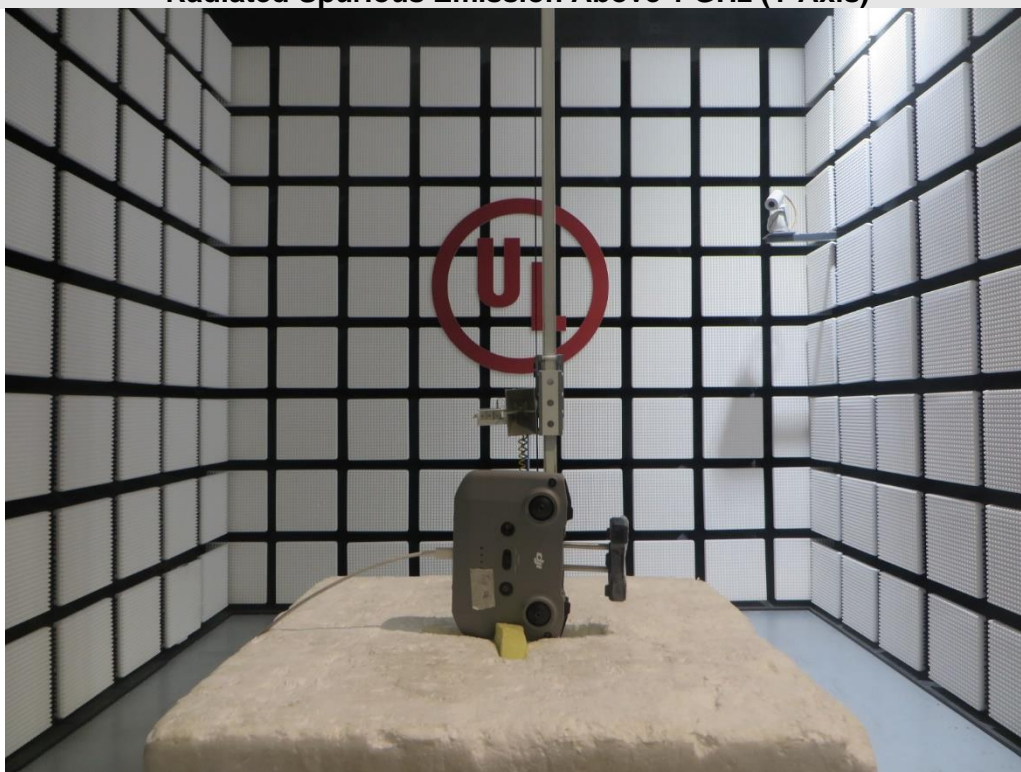
Radiated Spurious Emission Above 1 GHz (Y Axis)
