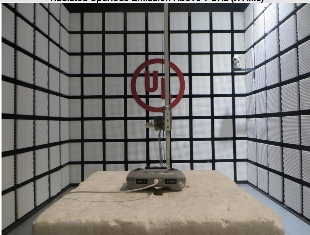
Radiated Spurious Emission Above 1 GHz (X Axis)
