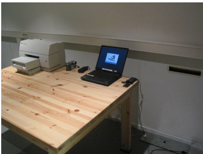
Picture 4 AC powerline conducted emission measurement GSM RX/WLAN TX + Computer peripherals
