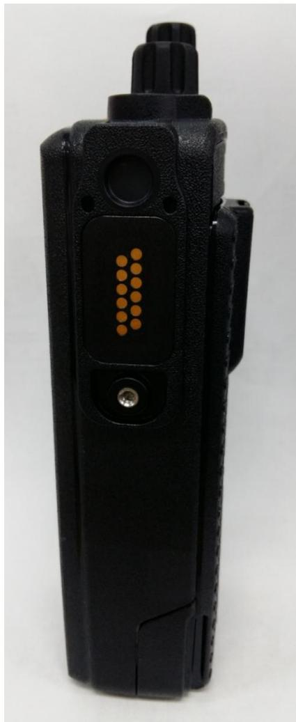
**Side View for Back View for Full Keypad and Non Keypad Models (Left)**
