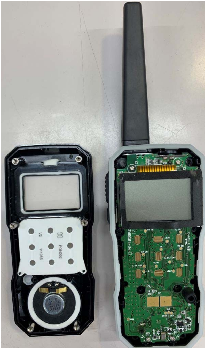
Figure E19.3 – Internal Photo – Front Cover Removed – Main PCB Display Side
