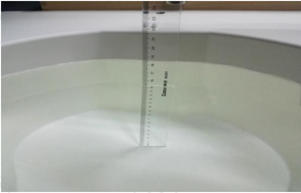
The Body Liquid of 2450MHz (15.3cm)
