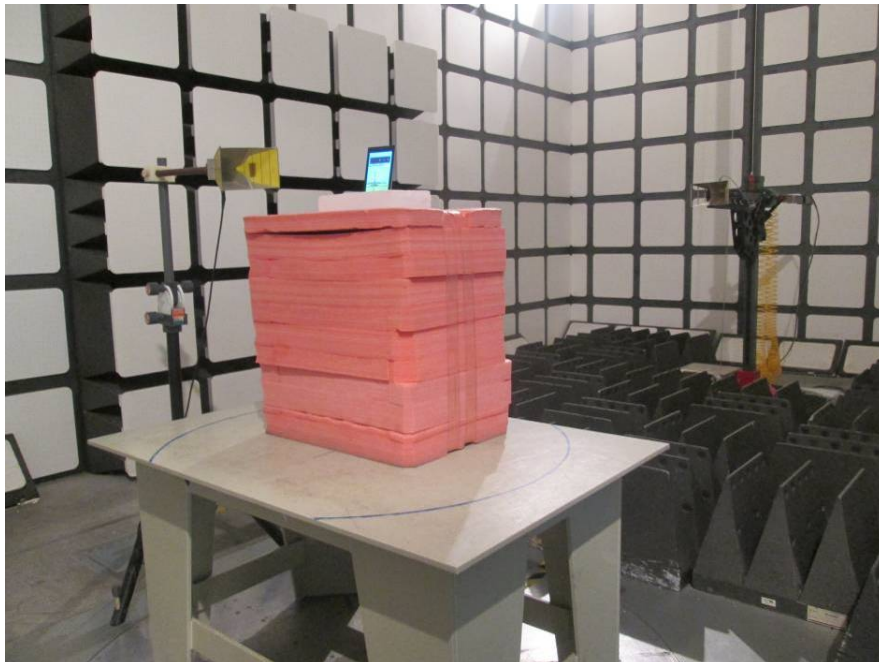
Radiated Emissions Test View (Above 1 GHz)
