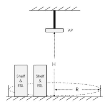
If multiple access points are needed, it is necessary to ensure that each access point signal has an overlapping area, and each label is at least within the coverage of more than one access point.
