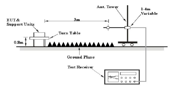
The radiated emission tests were performed in the 3 meters chamber test site, using the setup accordance with the ANSI C63.4-2014. The specification used was the FCC Part 15.109 Class B limits.
