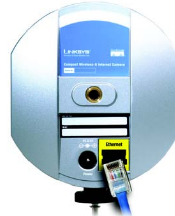
Figure 4-1: Connect the Ethernet Network Cable
