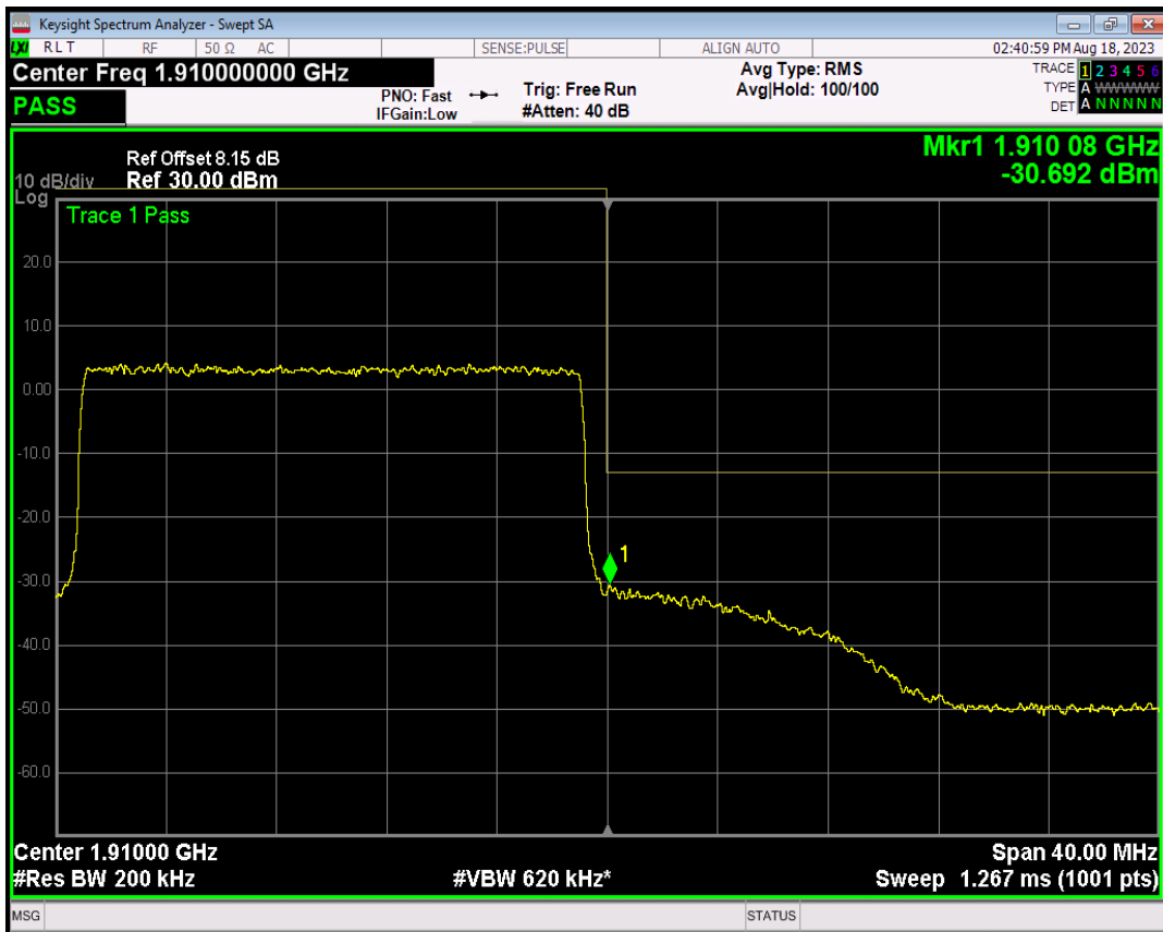
Band4 QPSK BW=1.4MHz Channel=19957 RB Size=1 Position=#0
