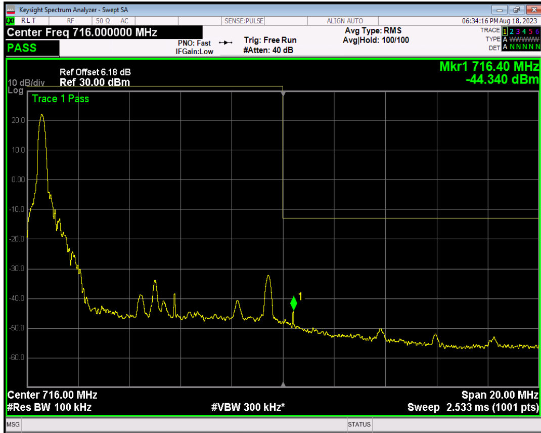
Band17 QPSK BW=10MHz Channel=23800 RB Size=1 Position=#Max
