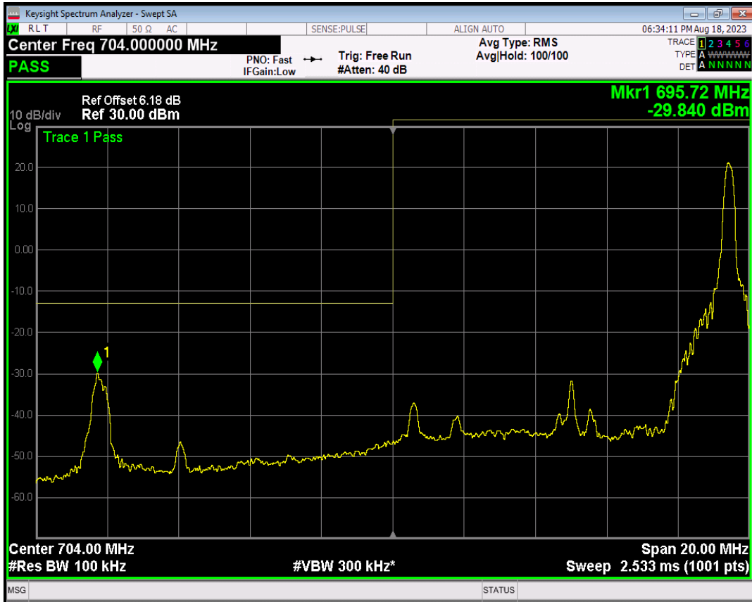
Band17 16QAM BW=10MHz Channel=23780 RB Size=50 Position=#0
