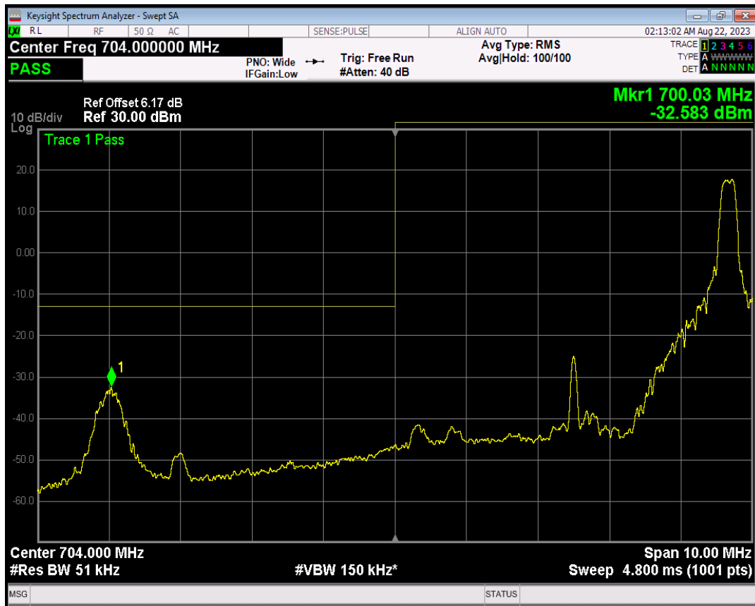
Band17 16QAM BW=5MHz Channel=23755 RB Size=25 Position=#0
