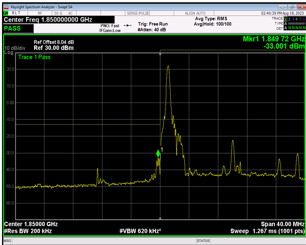
Band2 16QAM BW=20MHz Channel=18700 RB Size=1 Position=#Max
