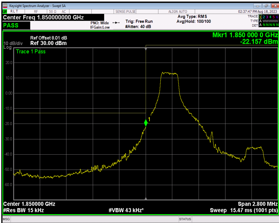
Band2 16QAM BW=1.4MHz Channel=18607 RB Size=1 Position=#Max
