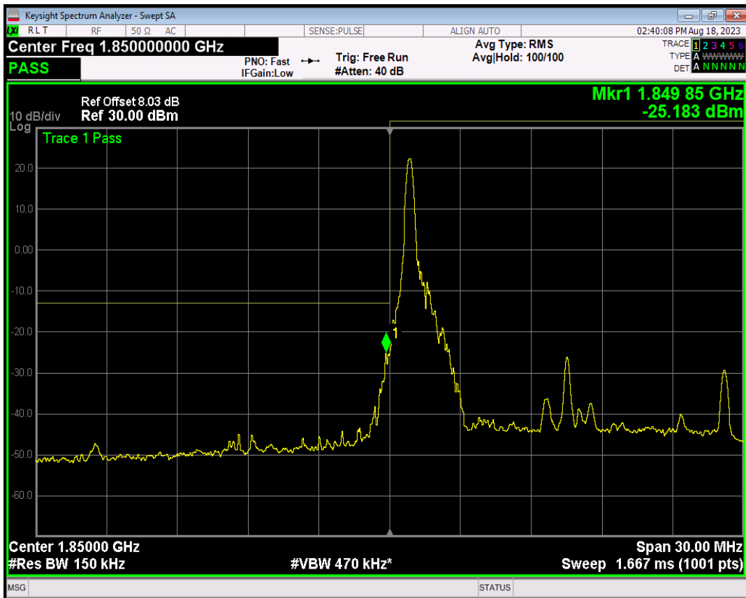
Band2 16QAM BW=15MHz Channel=18675 RB Size=1 Position=#Max
