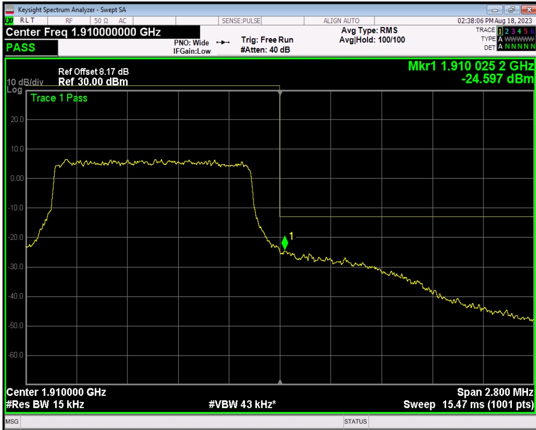
Band2 16QAM BW=1.4MHz Channel=19193 RB Size=1 Position=#0
