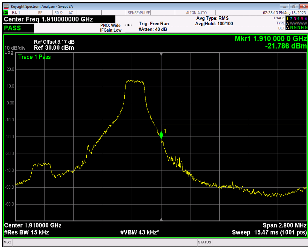
Band2 16QAM BW=1.4MHz Channel=19193 RB Size=6 Position=#0
