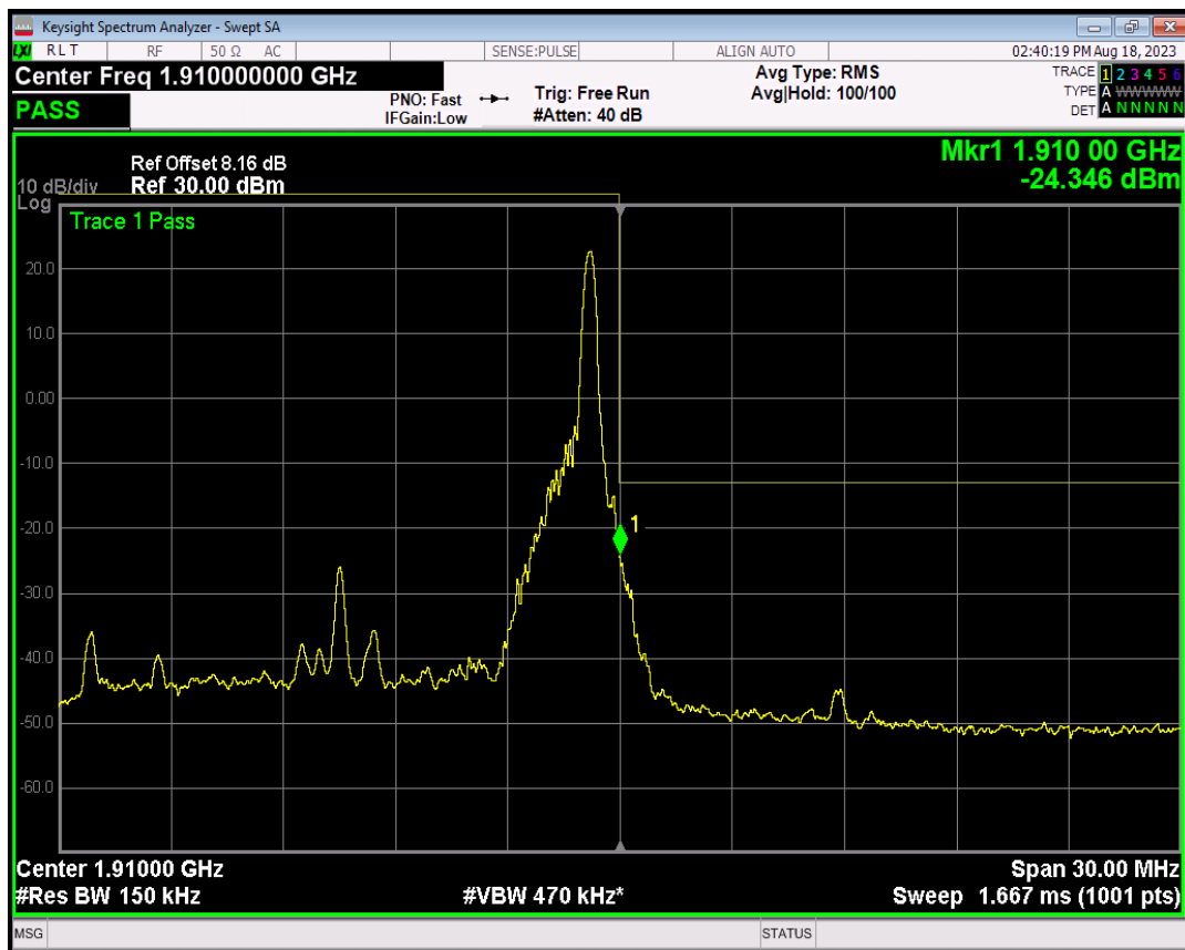
Band2 QPSK BW=15MHz Channel=19125 RB Size=75 Position=#0
