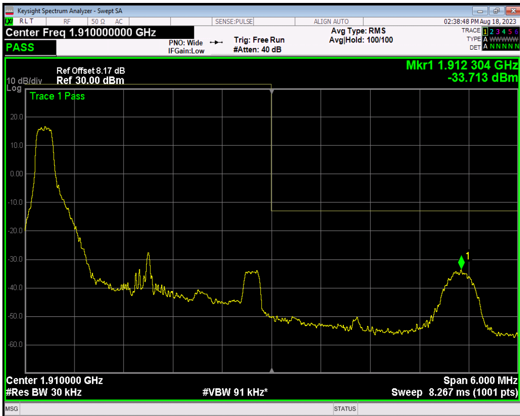
Band2 16QAM BW=3MHz Channel=19185 RB Size=1 Position=#Max
