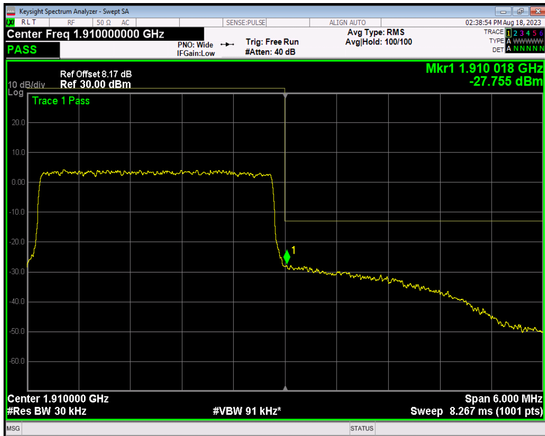
Band2 QPSK BW=5MHz Channel=18625 RB Size=1 Position=#0
