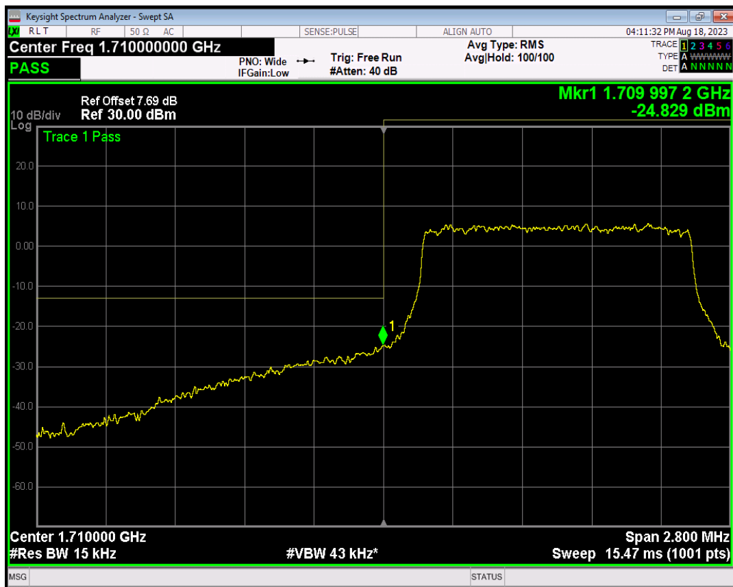
Band4 QPSK BW=1.4MHz Channel=20393 RB Size=1 Position=#0
