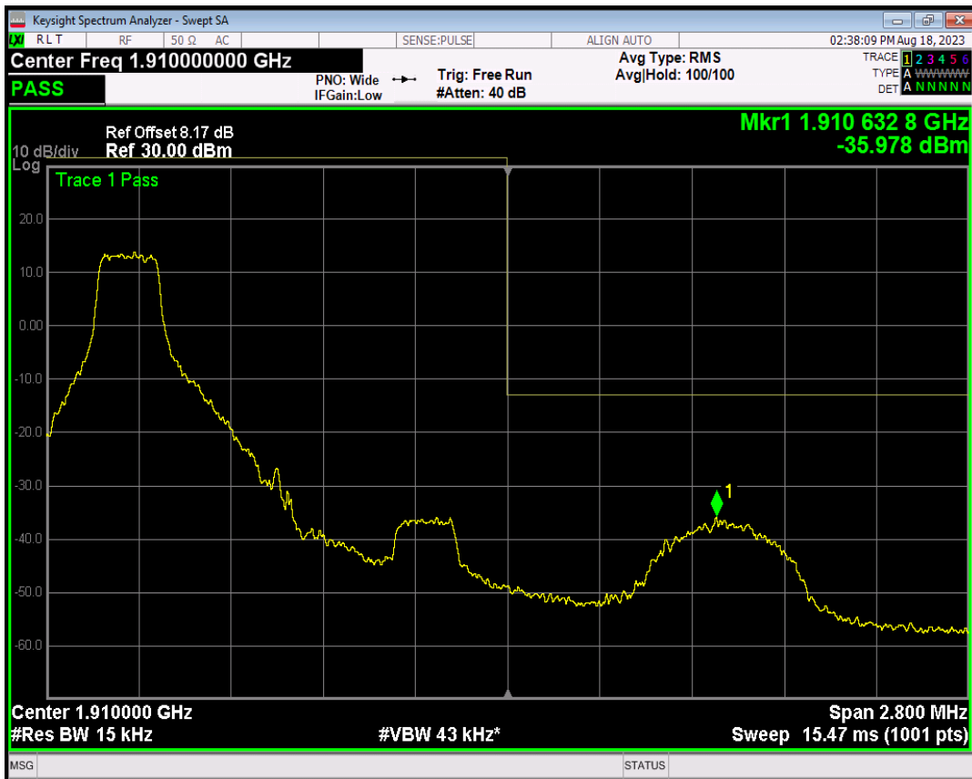
Band2 16QAM BW=1.4MHz Channel=19193 RB Size=1 Position=#Max
