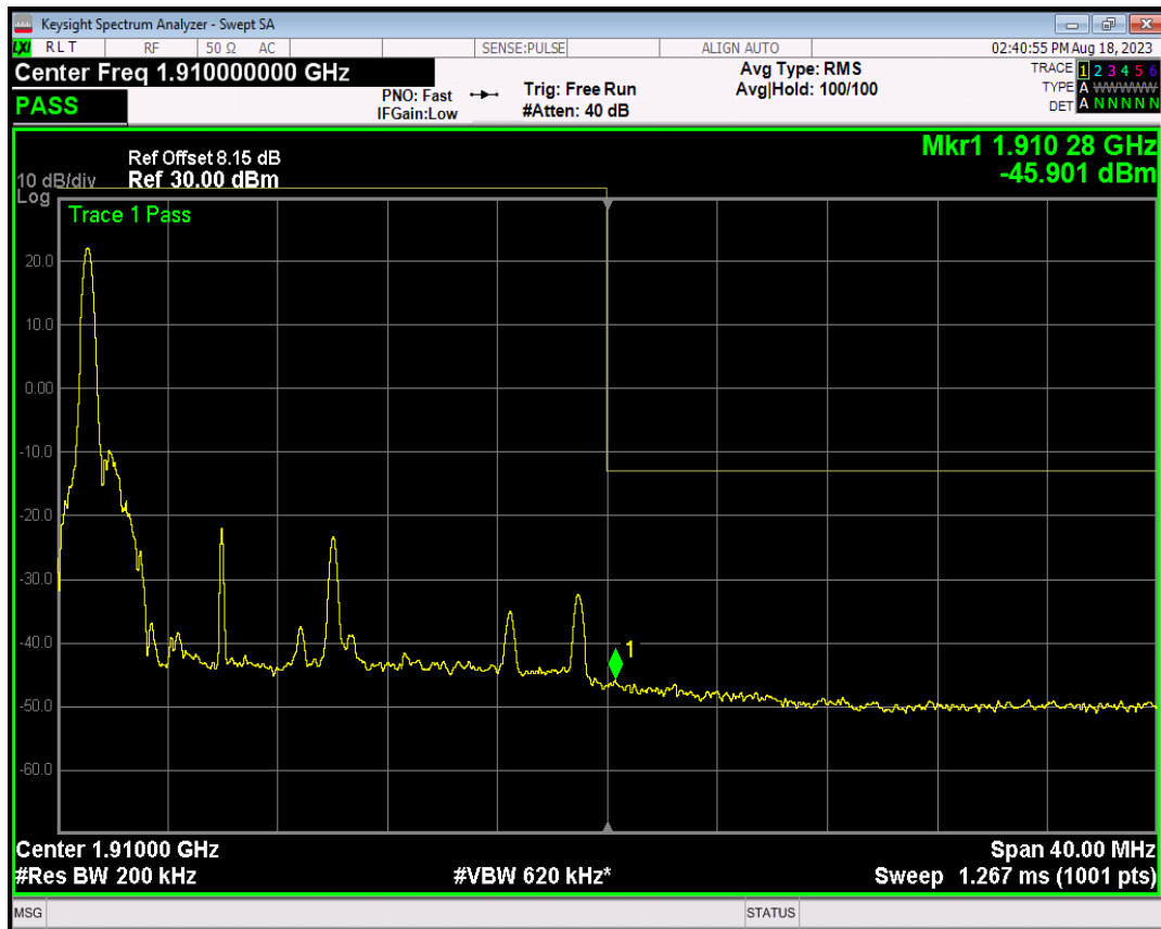
Band2 16QAM BW=20MHz Channel=19100 RB Size=1 Position=#Max
