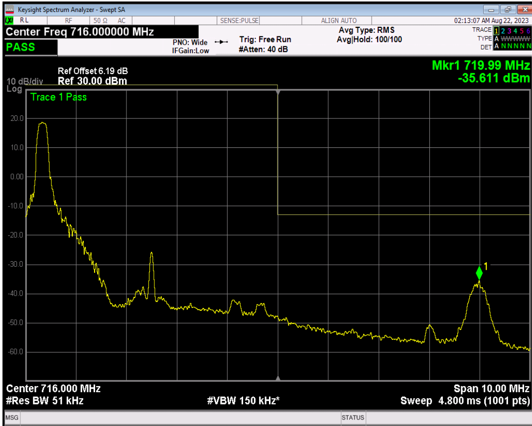
Band17 QPSK BW=5MHz Channel=23825 RB Size=1 Position=#Max
