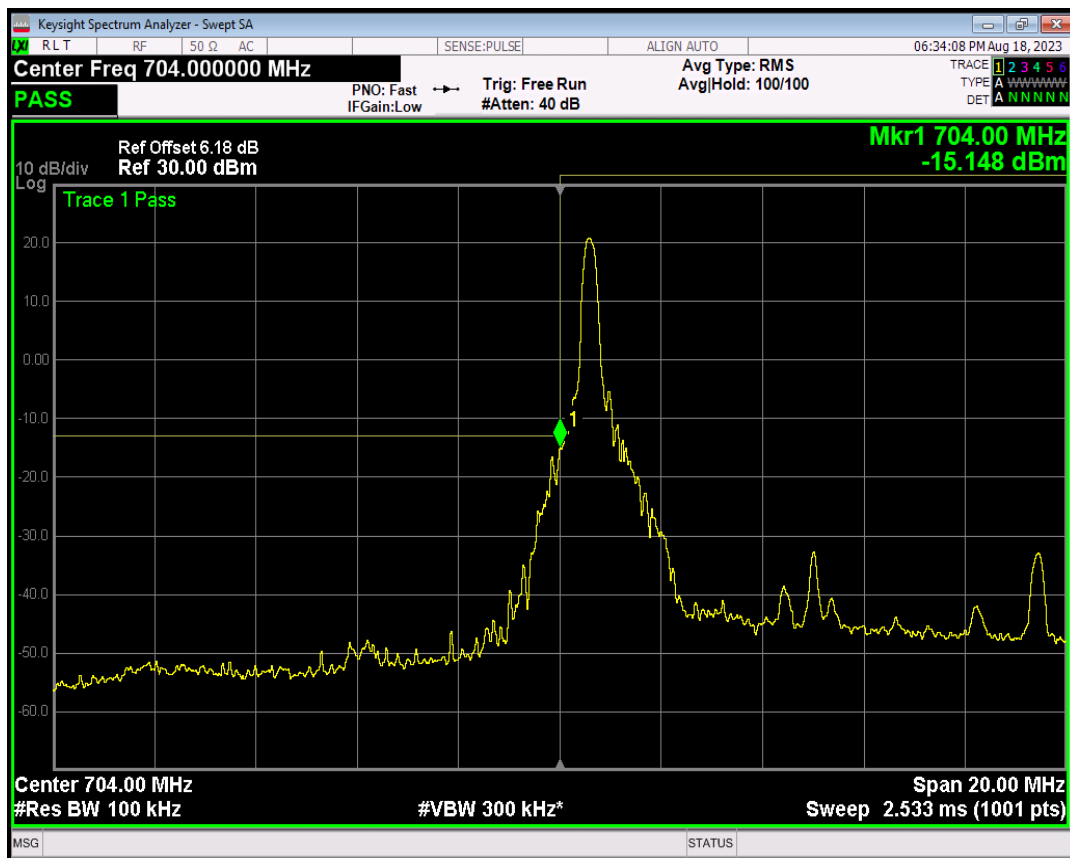
Band17 16QAM BW=10MHz Channel=23780 RB Size=1 Position=#Max
