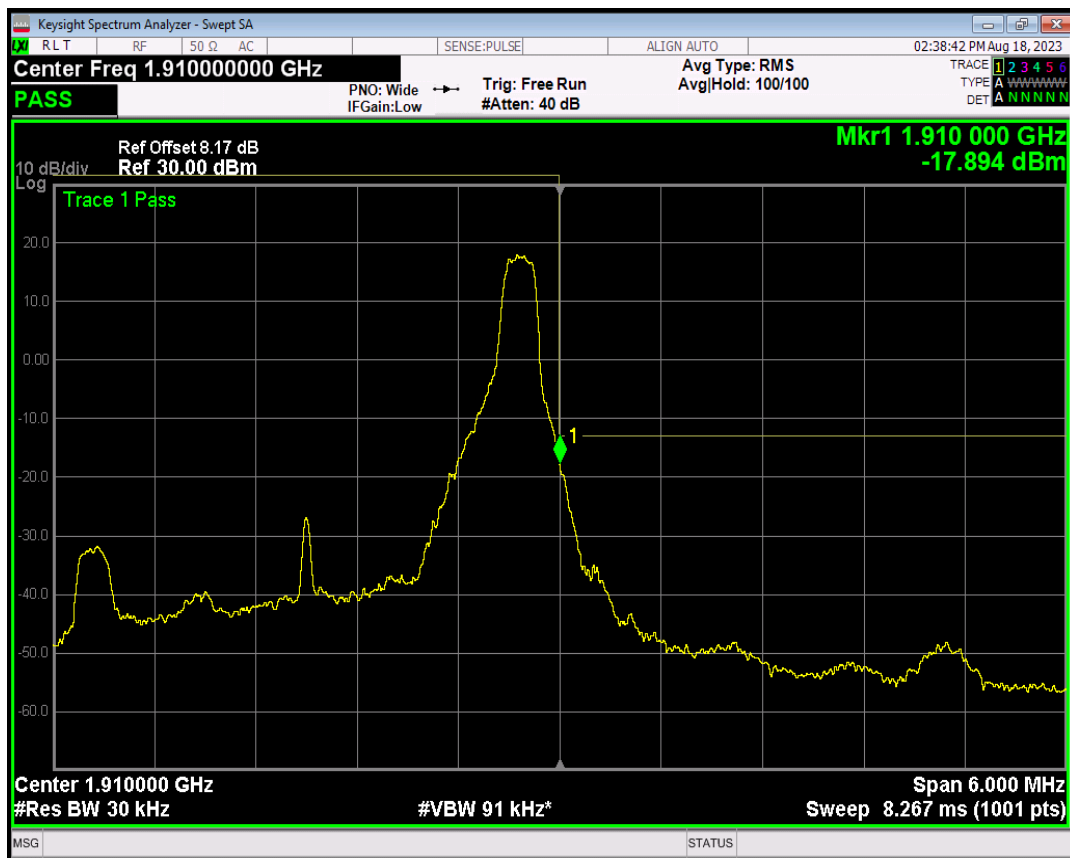
Band2 QPSK BW=3MHz Channel=19185 RB Size=15 Position=#0
