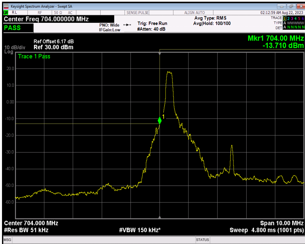
Band17 16QAM BW=5MHz Channel=23755 RB Size=1 Position=#Max
