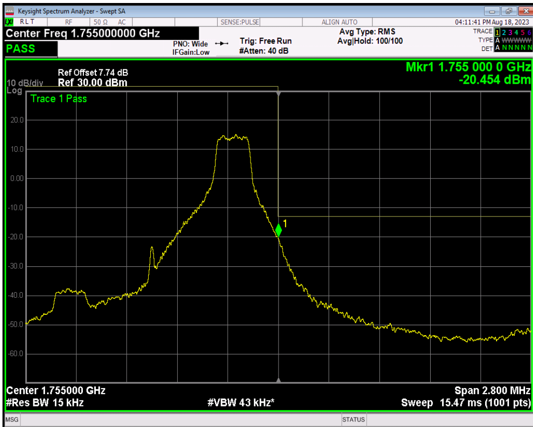
Band4 QPSK BW=1.4MHz Channel=20393 RB Size=6 Position=#0
