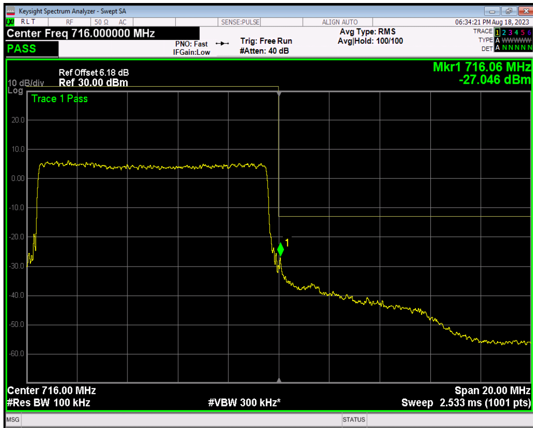
Band17 16QAM BW=10MHz Channel=23800 RB Size=1 Position=#0
