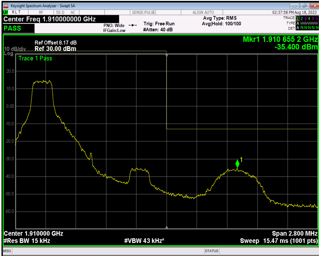
Band2 QPSK BW=1.4MHz Channel=19193 RB Size=1 Position=#Max
