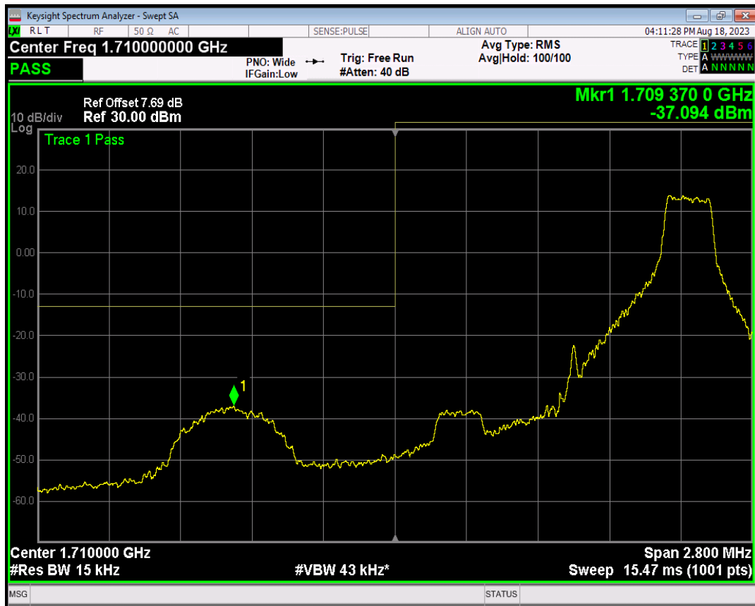
Band4 16QAM BW=1.4MHz Channel=19957 RB Size=6 Position=#0
