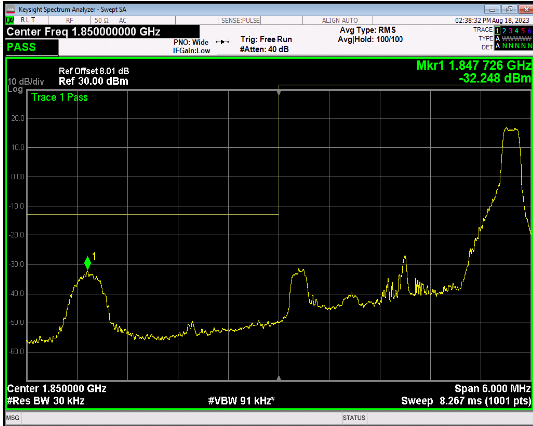
Band2 16QAM BW=3MHz Channel=18615 RB Size=15 Position=#0
