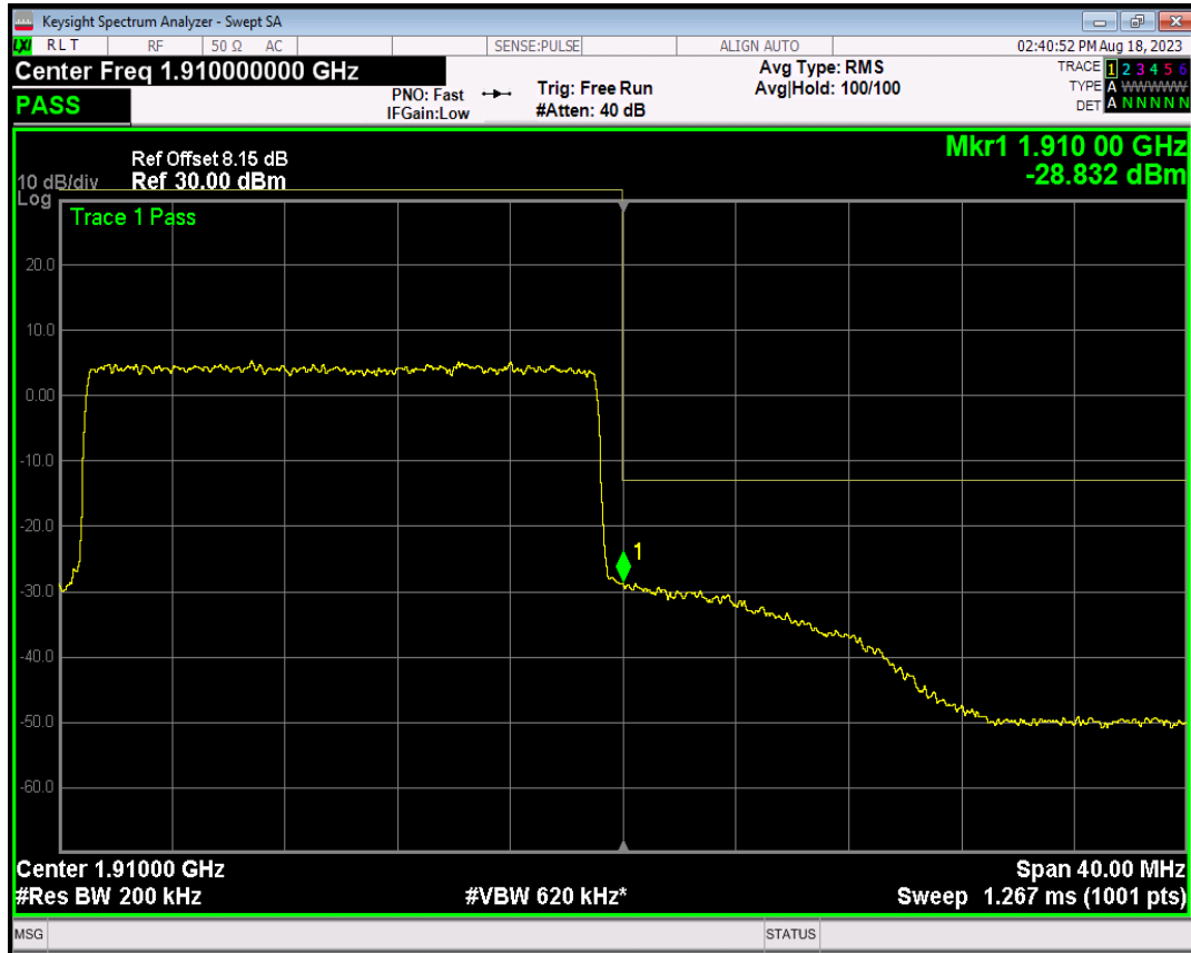
Band2 16QAM BW=20MHz Channel=19100 RB Size=1 Position=#0
