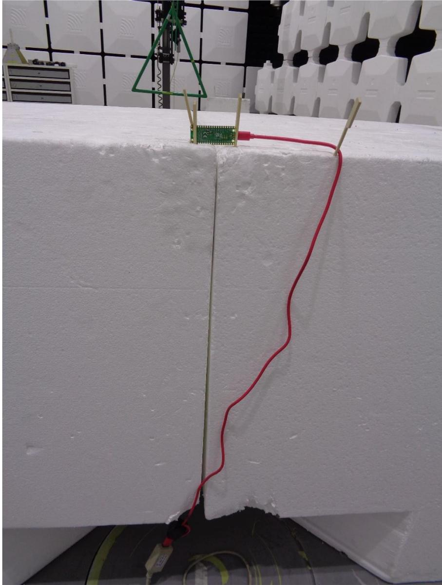
**Positioning of Wurth 742 711 31 S ferrite on USB cable**
