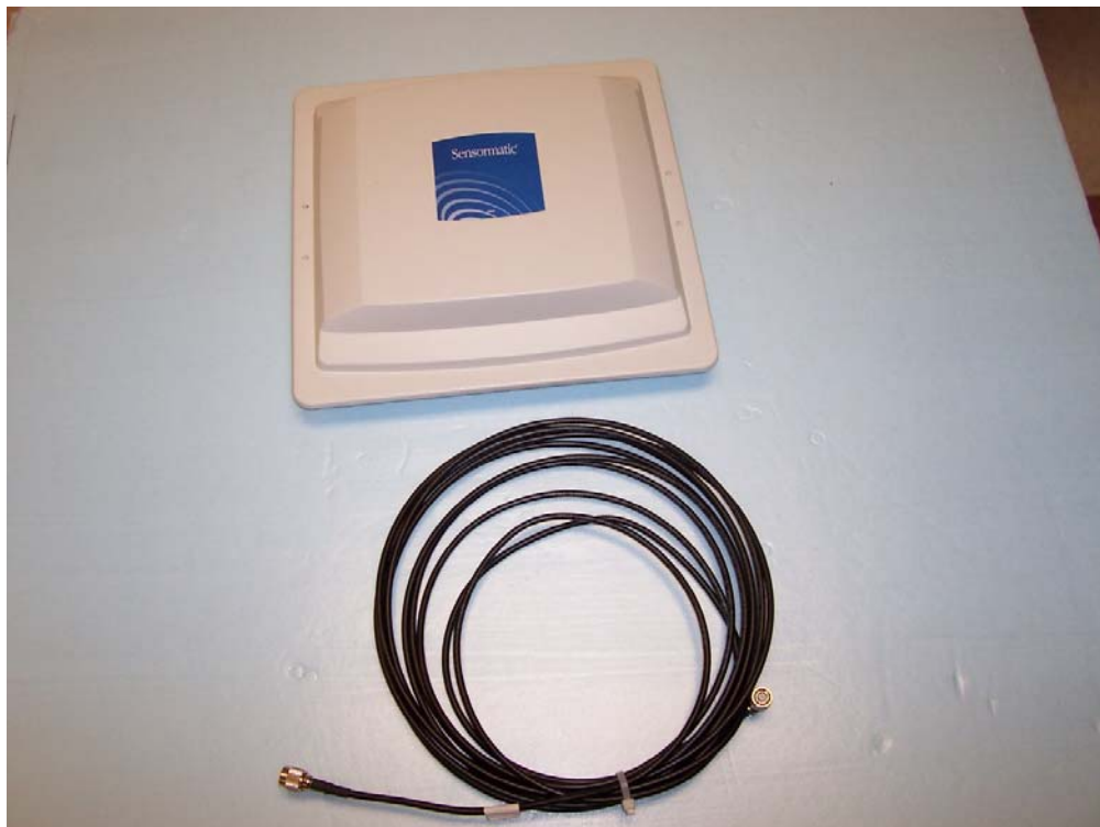
OmniWave Antenna with supplied 25' coaxial cable
