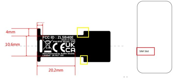
Note: This label is placed above SIM booth. The yellow stop it falling out. So the label can not fall our in fact.
