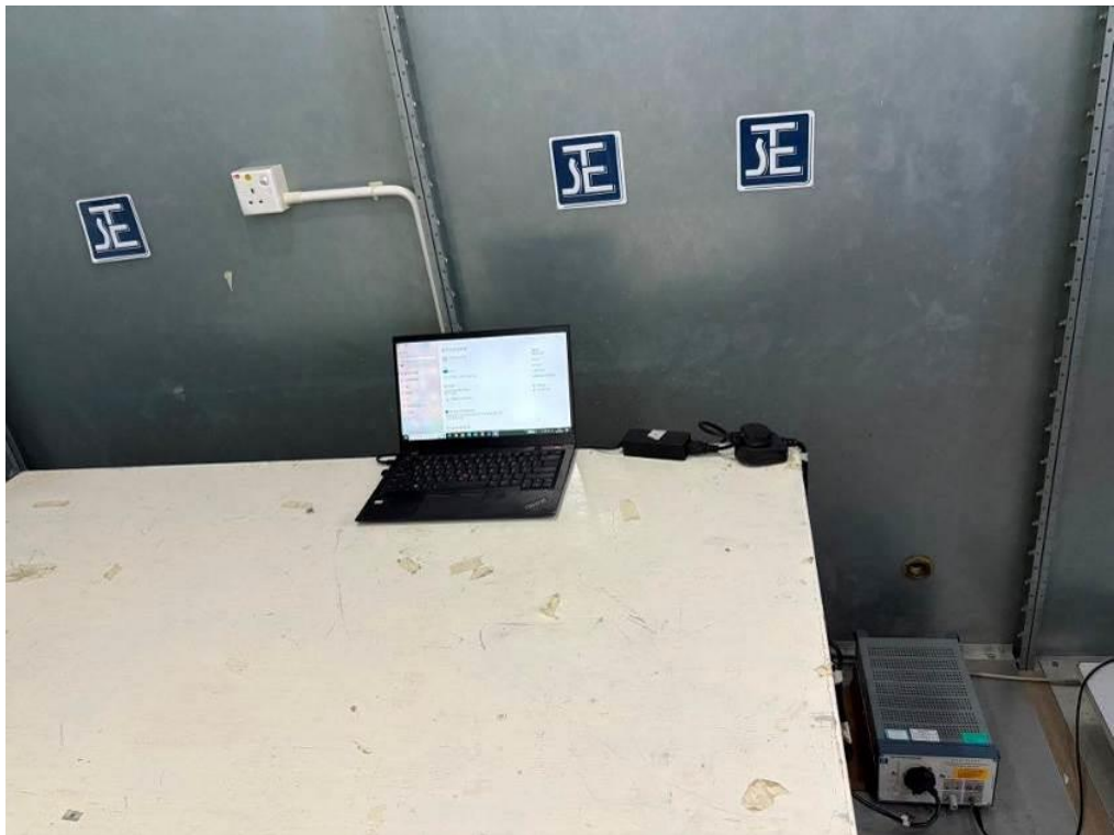
Measurement of Conducted Emission Test Set Up
