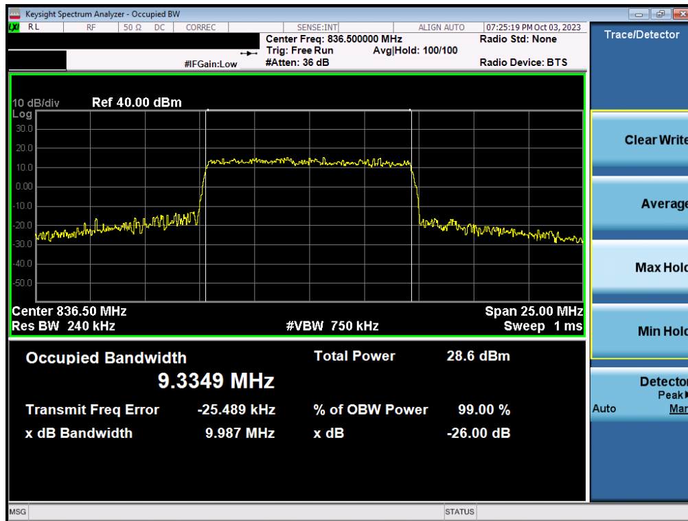
Plot 7-19. Occupied Bandwidth Plot (NR Band n5 - 10MHz 16-QAM - Full RB)
