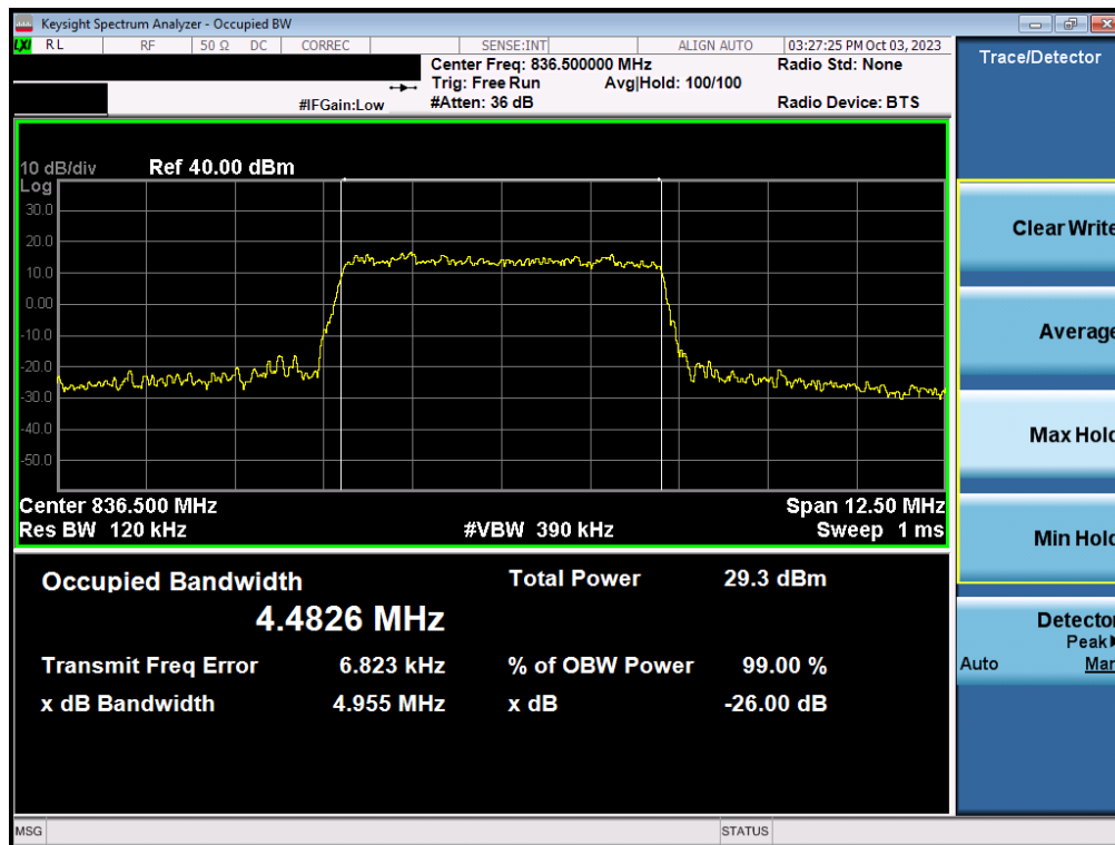
Plot 7-6. Occupied Bandwidth Plot (LTE Band 26/5 - 5MHz 16-QAM - Full RB)
