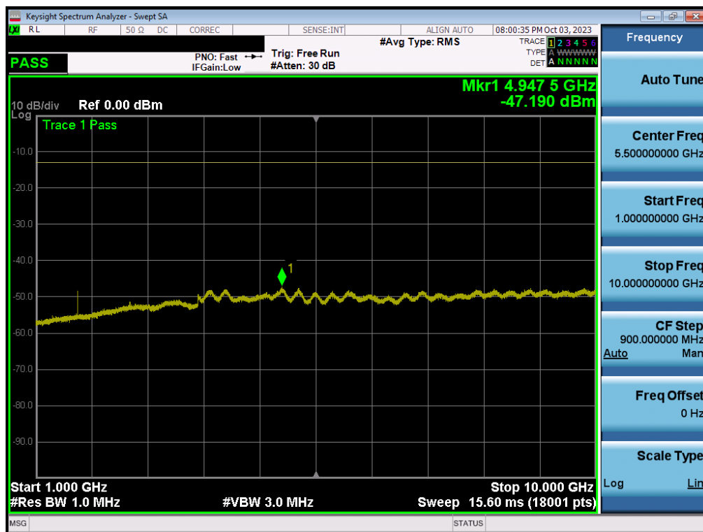
Plot 7-31. Conducted Spurious Plot (NR Band n5 - 20.0MHz - 1 RB - Mid Channel)
