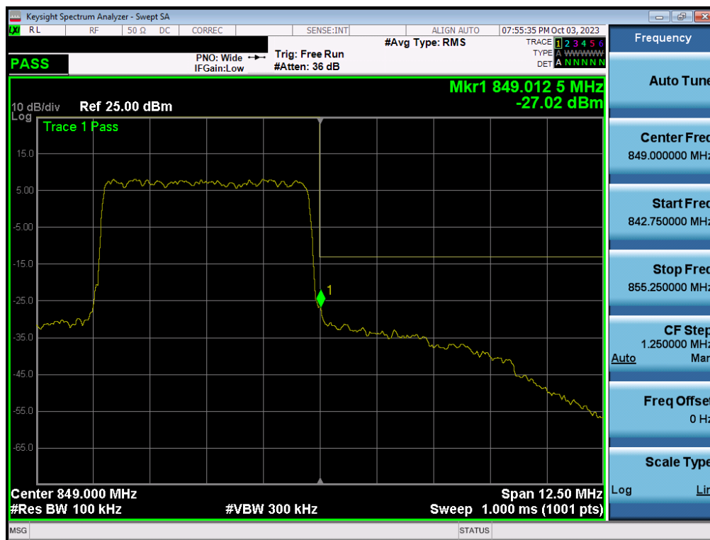
Plot 7-41. Upper Band Edge Plot (NR Band n5 – 5.0MHz - Full RB)
