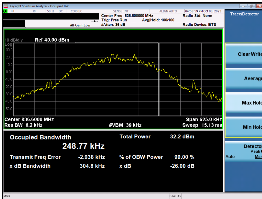
Plot 7-24. Occupied Bandwidth Plot (EDGE, Ch. 190)
