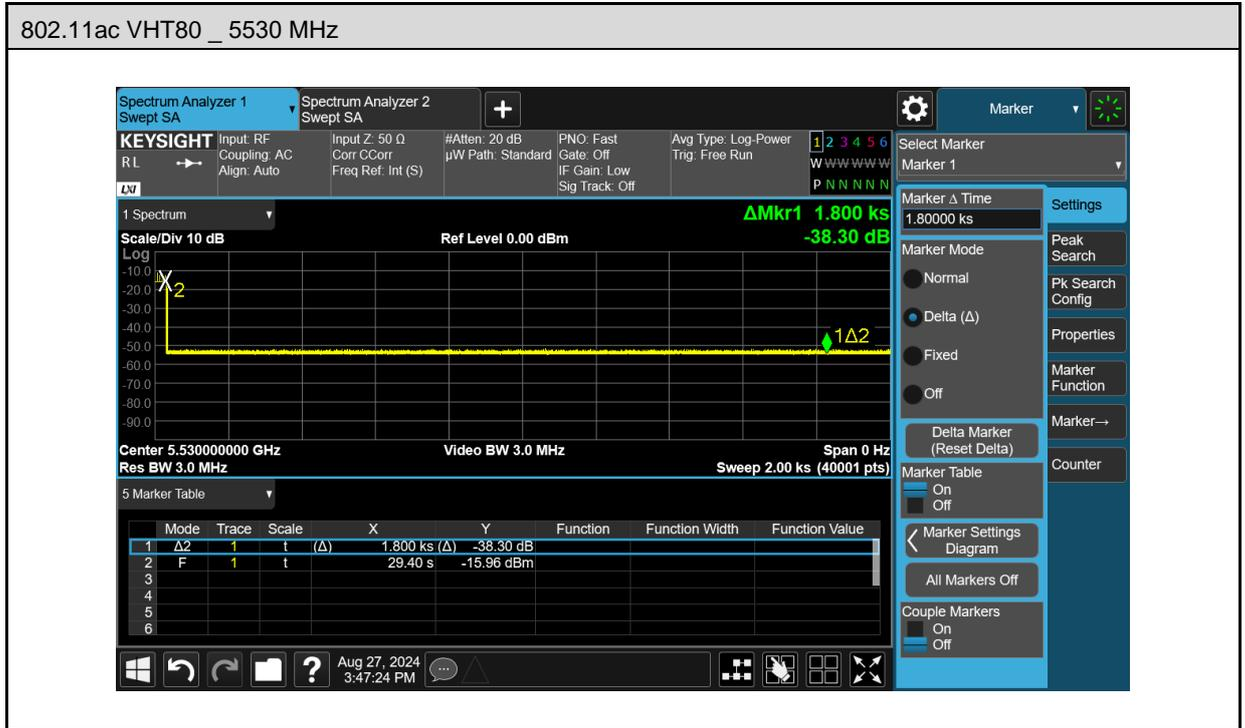
Note: Non-Occupancy Period time is 30 minute during which a Channel will not be utilized after a Radar Waveform is detected on that Channel.
