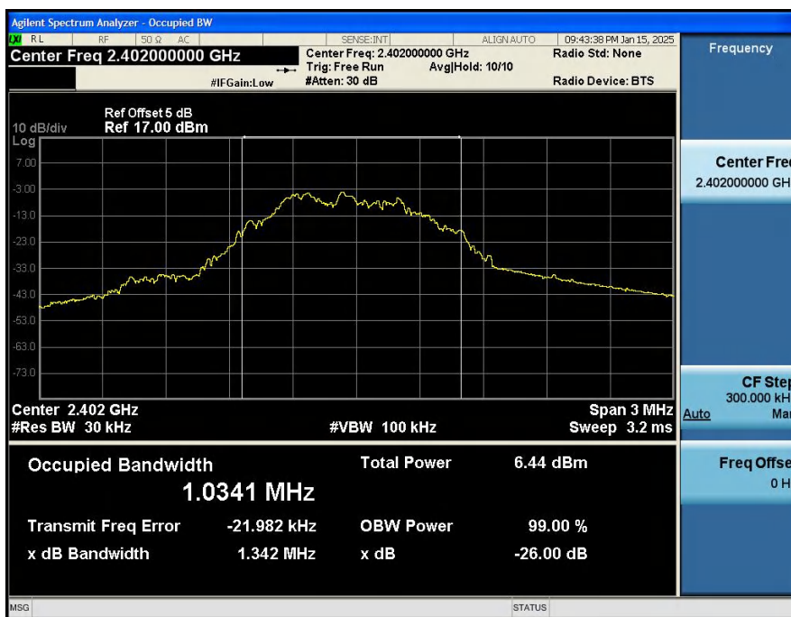
99%_Occupied_Bandwidth_NVNT_ANT1_1Mbps_2402
