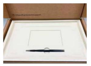
Locate the Framework Screwdriver in the package underneath the Framework Laptop and keep it handy - it's the only tool you'll need if you ever want to upgrade or replace any of the components in your Framework Laptop!
