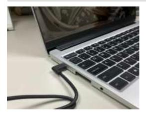
Plug in the charger into the USB-C Expansion Card and then connect the AC Cable to a power source.
