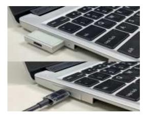
• It is highly recommended you insert a USB-C Expansion Card into the Framework Laptop since it is difficult to directly plug a charger into the recessed USB-C receptacle that is inside the bay.
