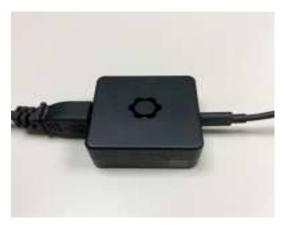
Assemble the modular Power Adapter. Connect the AC cable and the USB-C cable to the Power Adapter.
