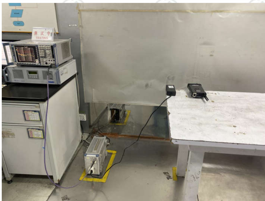
Conducted Emissions Test Setup
