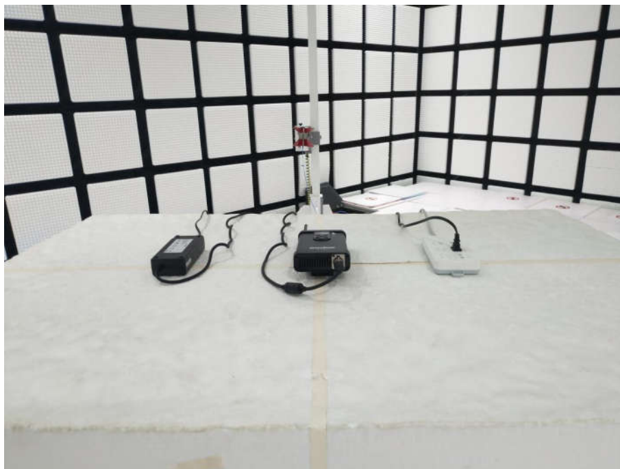
Radiated spurious emission Test Setup-3(Above 1GHz)
