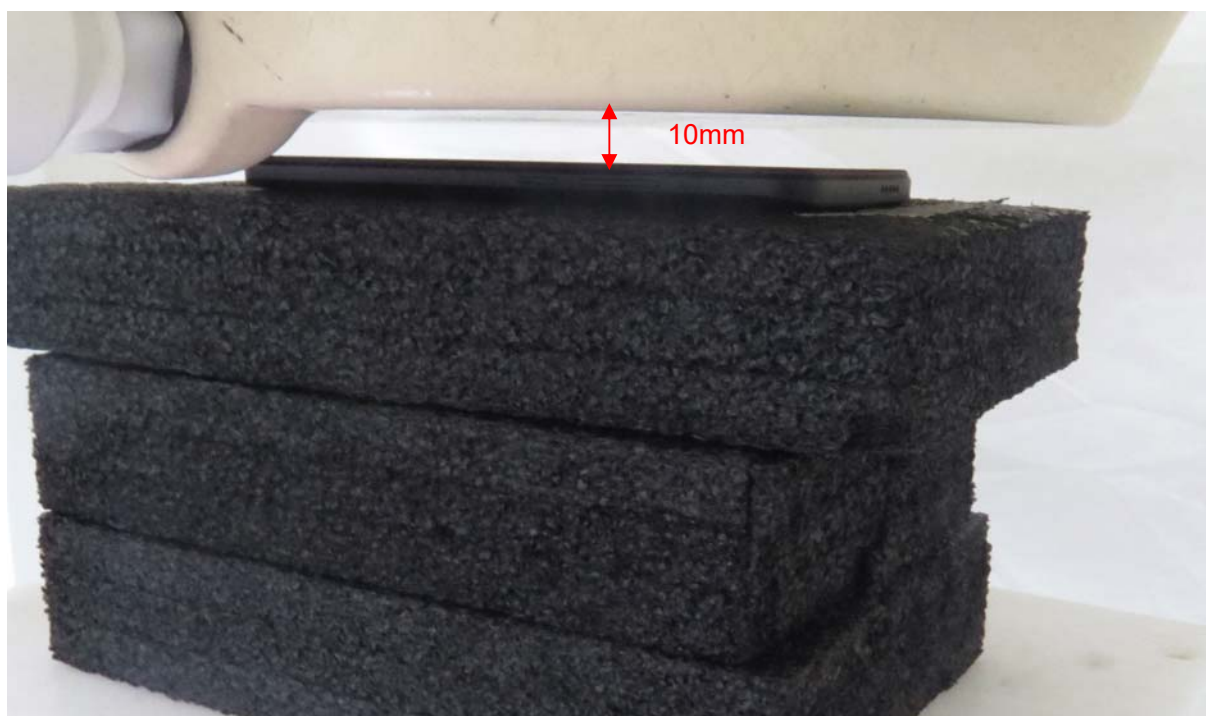
Picture 8: Front Side, the distance from handset to the bottom of the Phantom is 10mm
