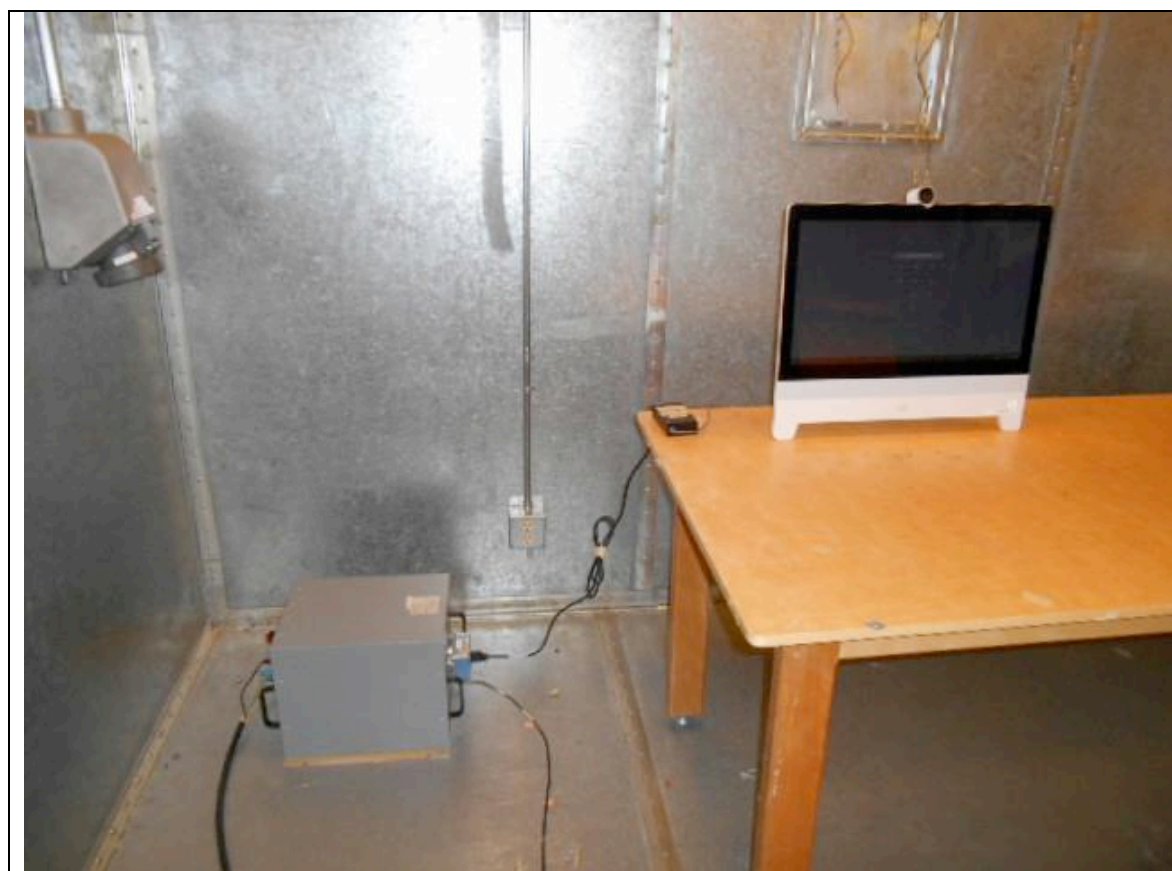
Title: Conducted Emissions Test Configuration
