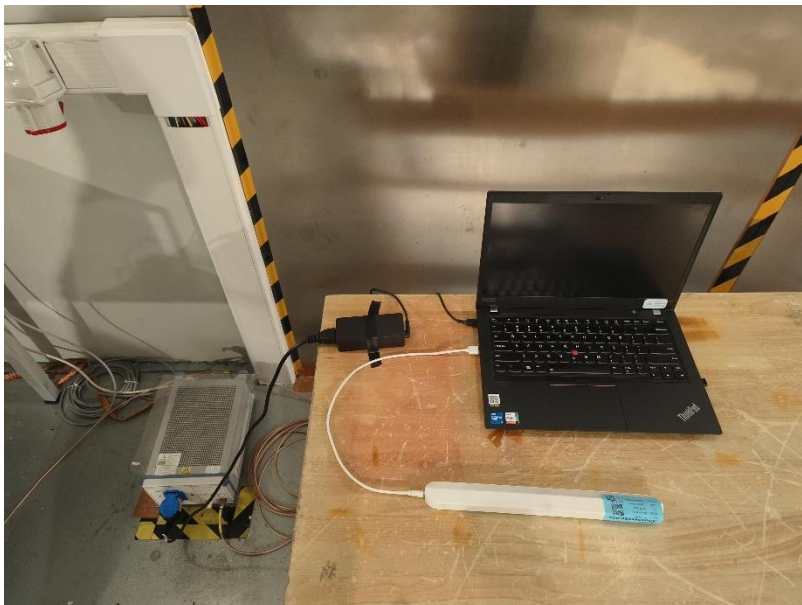
Photograph 2: Set-up for measurement of conducted emission, Mode 2
