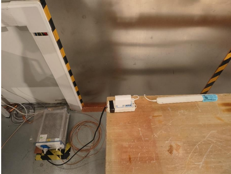
Photograph 2: Set-up for measurement of conducted emission, Mode 2
